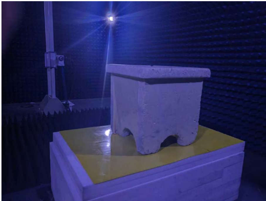
Photo of Radiated Emission Measurement Above 1GHz
