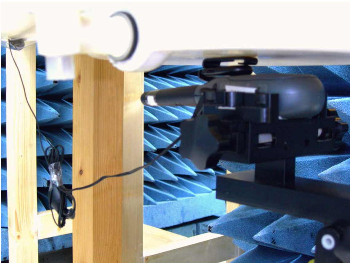
Figure15. SAR Test Setup w/Belt Clip
