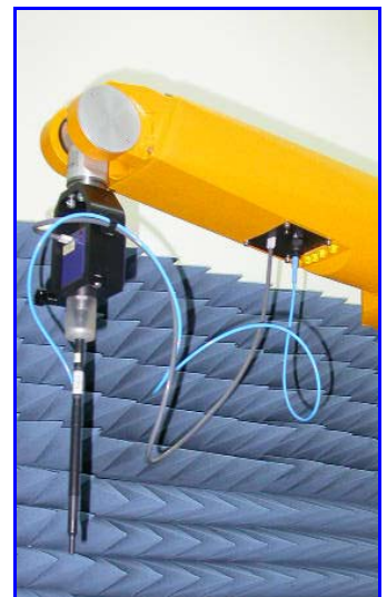
Figure 7. Probe setup on robot
