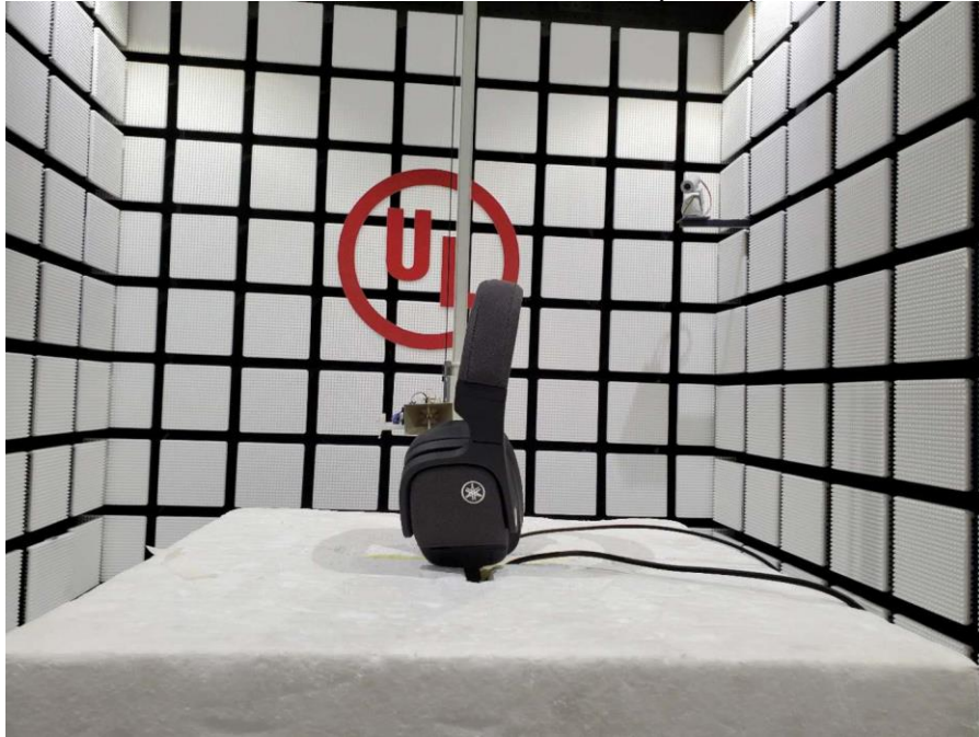
RADIATED RF MEASUREMENT SETUP (30MHz~1GHz)
