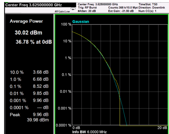
Channel: MIDDLE, Modulation: 16QAM, BW=5MHz, CCDF
