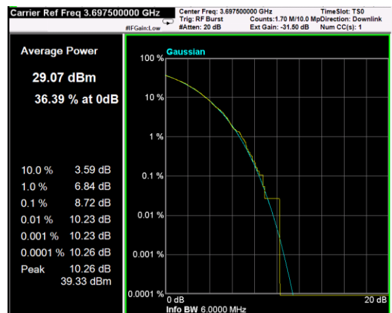
Channel: TOP, Modulation: QPSK, BW=5MHz, CCDF
