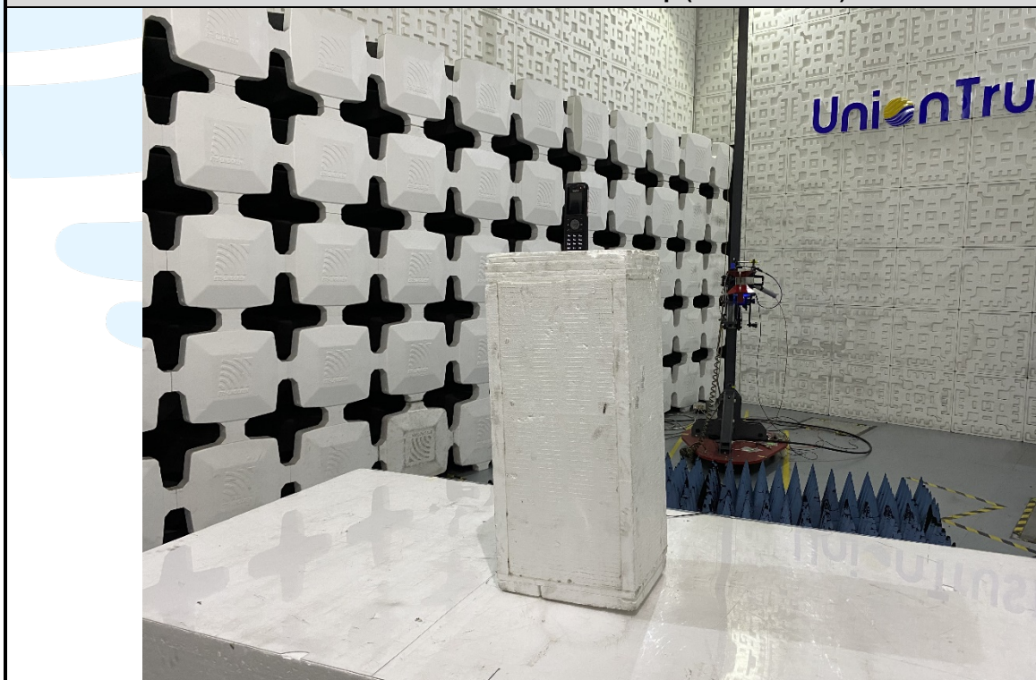
Radiated emission Test Setup (Above 1 GHz)
