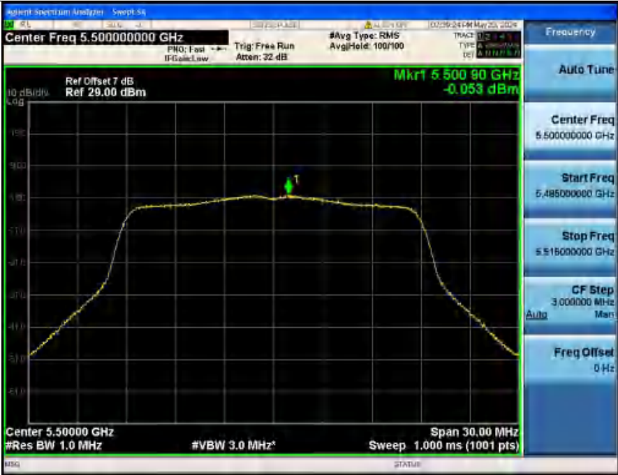
Power Spectral Density NVNT ANT2_802_11n(HT20)_5500
