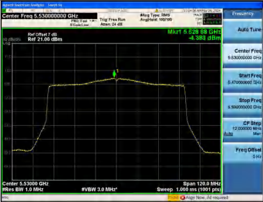
Power Spectral Density NVNT_ANT2_802_11ax(HE80)_5530
