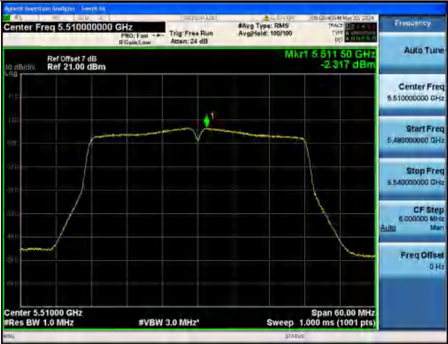
Power Spectral Density NVNT ANT2_802_11n(HT40)_5510
