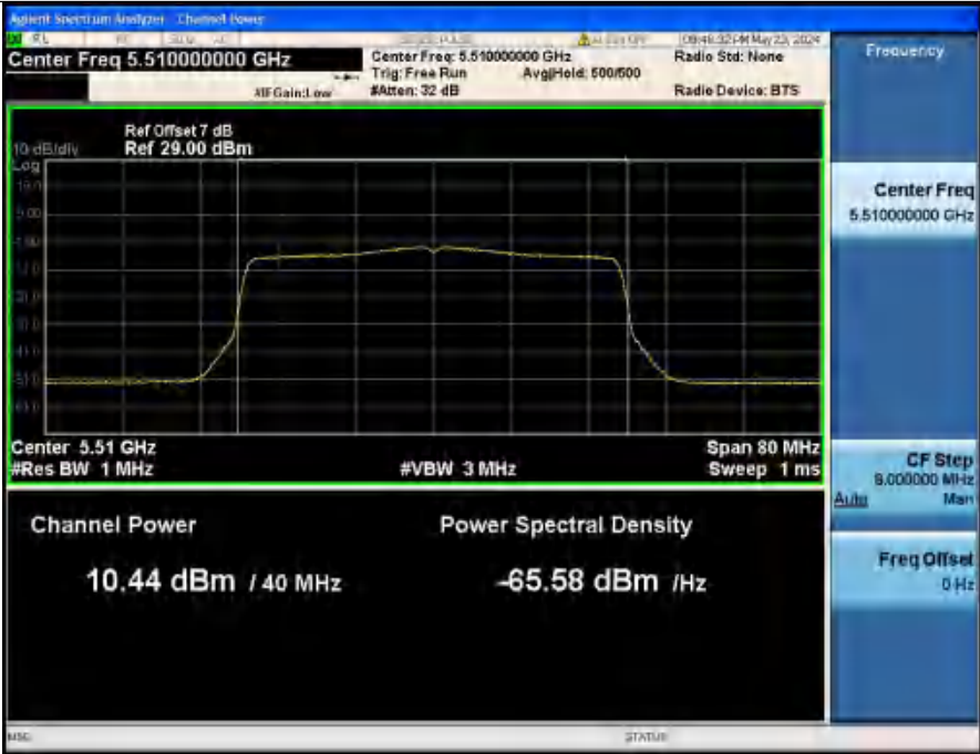
Maximum Conducted Output Power NVNT_ANT2_802_11ax(HE40)_5510_40M
