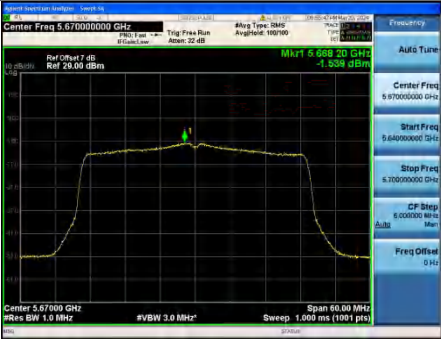
Power Spectral Density NVNT_ANT2_802_11ax(HE40)_5670
