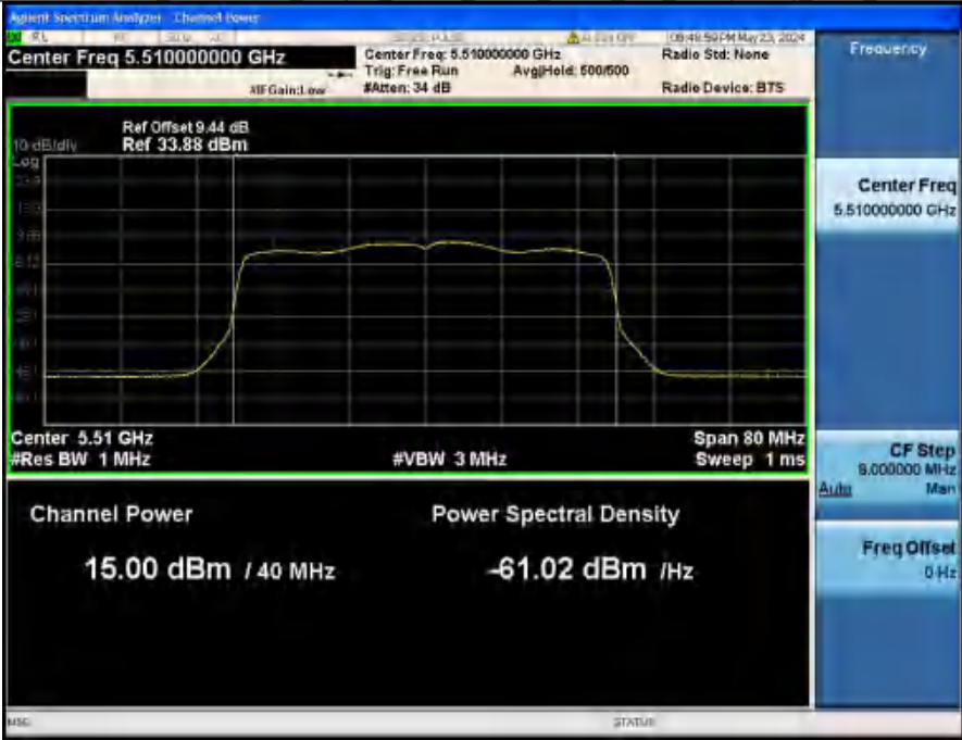
Maximum Conducted Output Power NVNT_ANT2_802_11ax(HE40)_5510_40M
