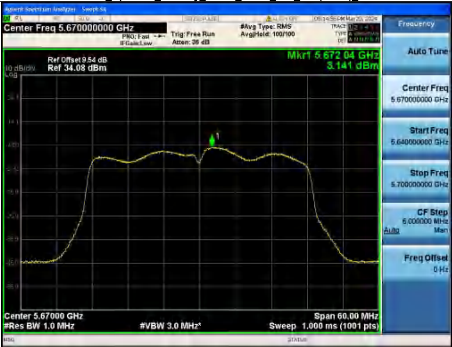
Power Spectral Density NVNT ANT2_802_11n(HT40)_5670
