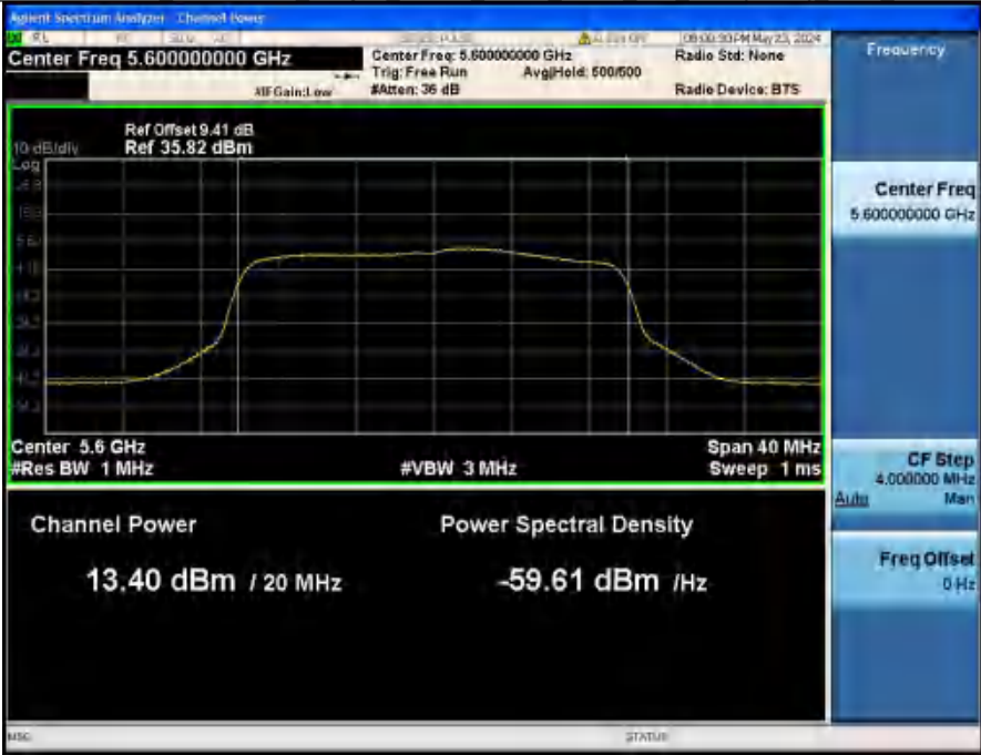
Maximum Conducted Output Power NVNT_ANT2_802_11ax(HE20)_5600_20M
