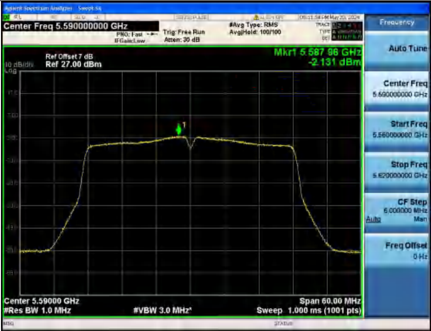
Power Spectral Density NVNT ANT2_802_11n(HT40)_5590
