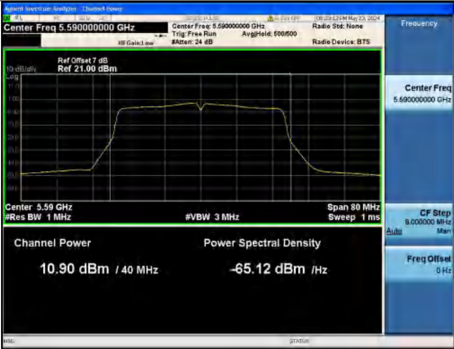
Maximum_Conducted_Output_Power_NVNT_ANT2_802_11ac(VHT40)_5590_40M
