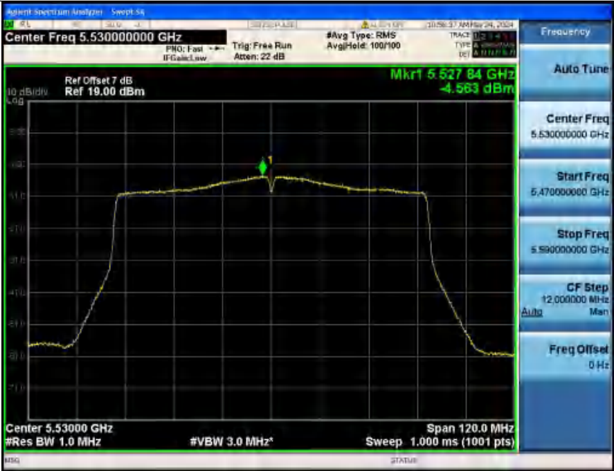
Power Spectral Density NVNT_ANT2_802_11ac(VHT80)_5530
