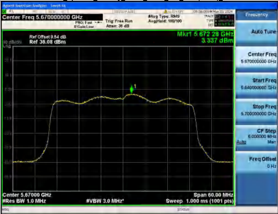
Power Spectral Density NVNT_ANT2_802_11ax(HE40)_5670
