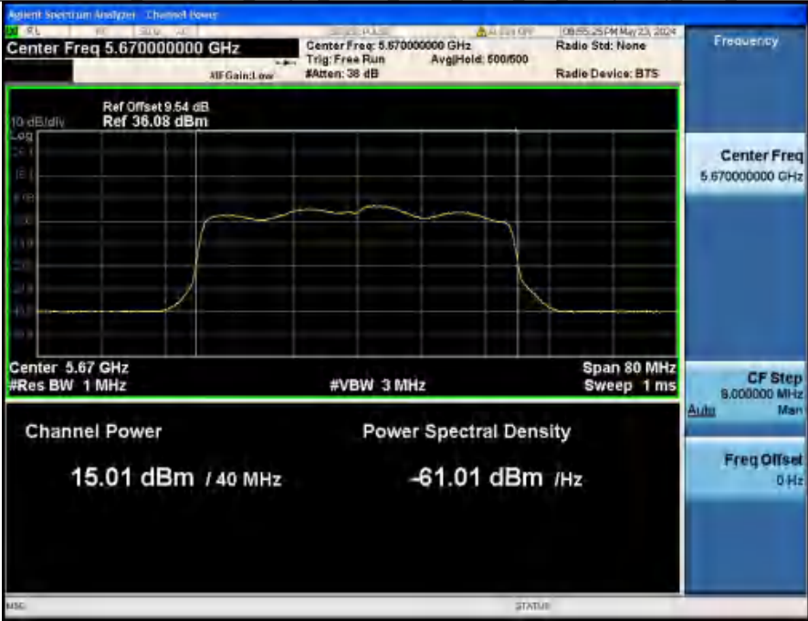
Maximum Conducted Output Power NVNT ANT2_802_11ax(HE40) 5670_40M
