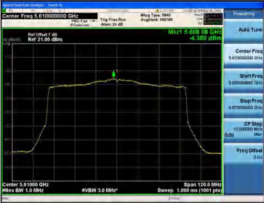
Power Spectral Density NVNT_ANT2_802_11ax(HE80)_5610
