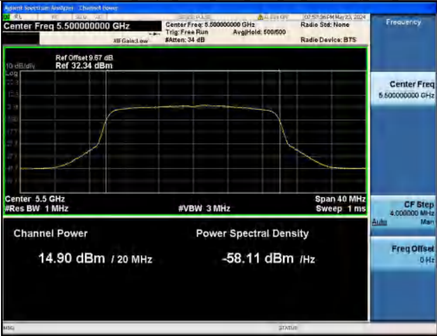
Maximum Conducted Output Power NVNT_ANT2_802_11ax(HE20)_5500_20M
