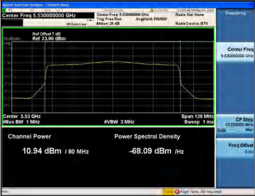
Maximum Conducted Output Power NVNT ANT2_802_11ax(HE80)_5530_80M
