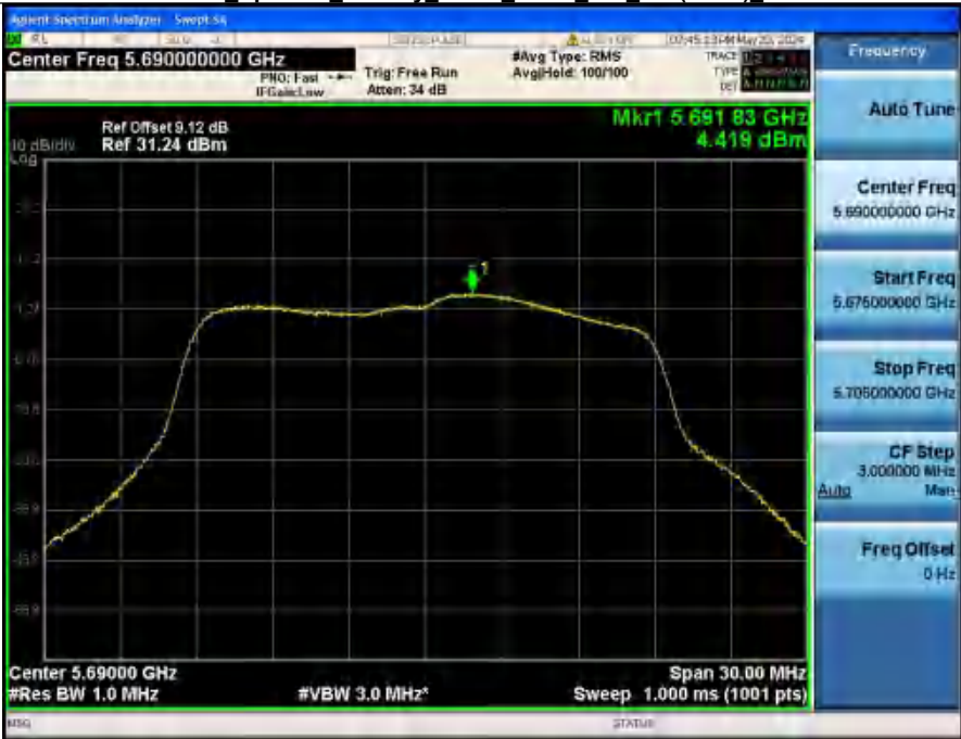
Power Spectral Density NVNT ANT2_802_11n(HT20)_5700
