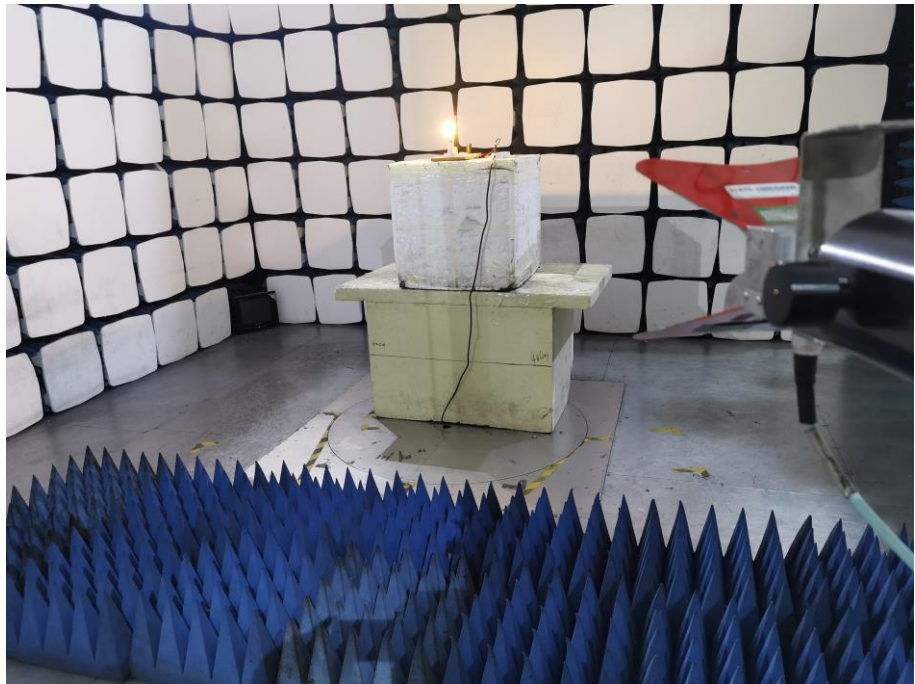
Radiation Emission Test Setup (1GHz to 18GHz)
