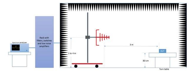
Radiated Setup 1 GHz - 18 GHz
