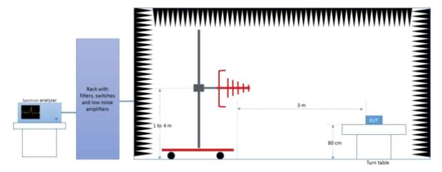
Radiated Setup 1 GHz - 18 GHz
