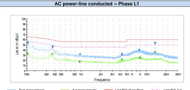
Limit FCC Quasi-Peak - · - · · Limit FCC Avg Peak measurements Avg measurements
