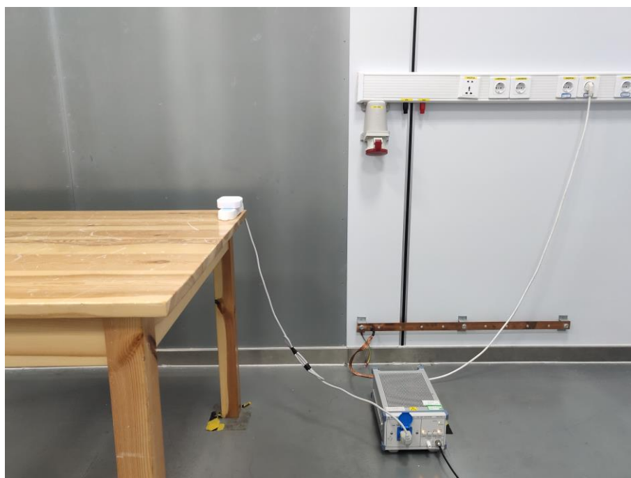
Fig. 4 Power line conducted emission setup photo
