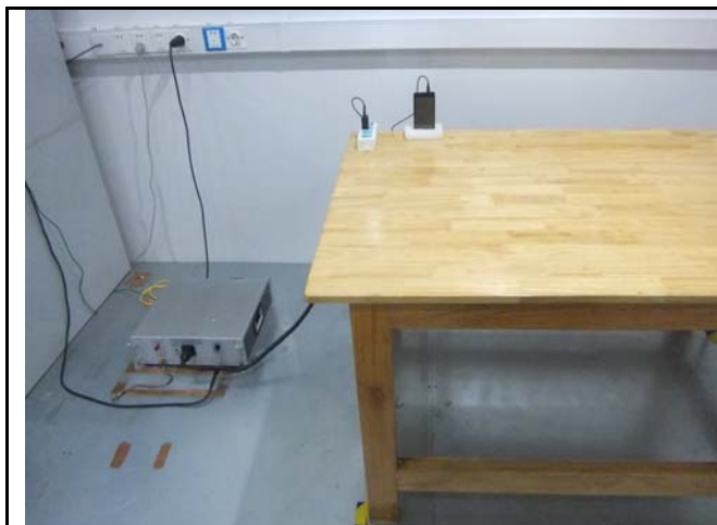
Conducted Emissions Test Setup Front View
