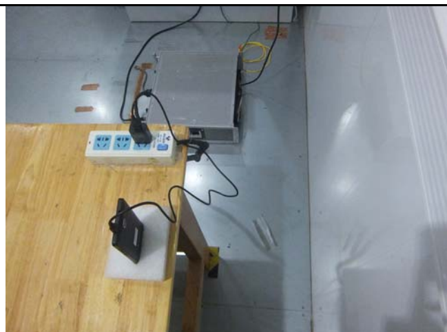
Conducted Emissions Test Setup Side View
