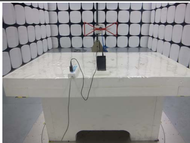
Conducted Emissions Test Setup Front View
