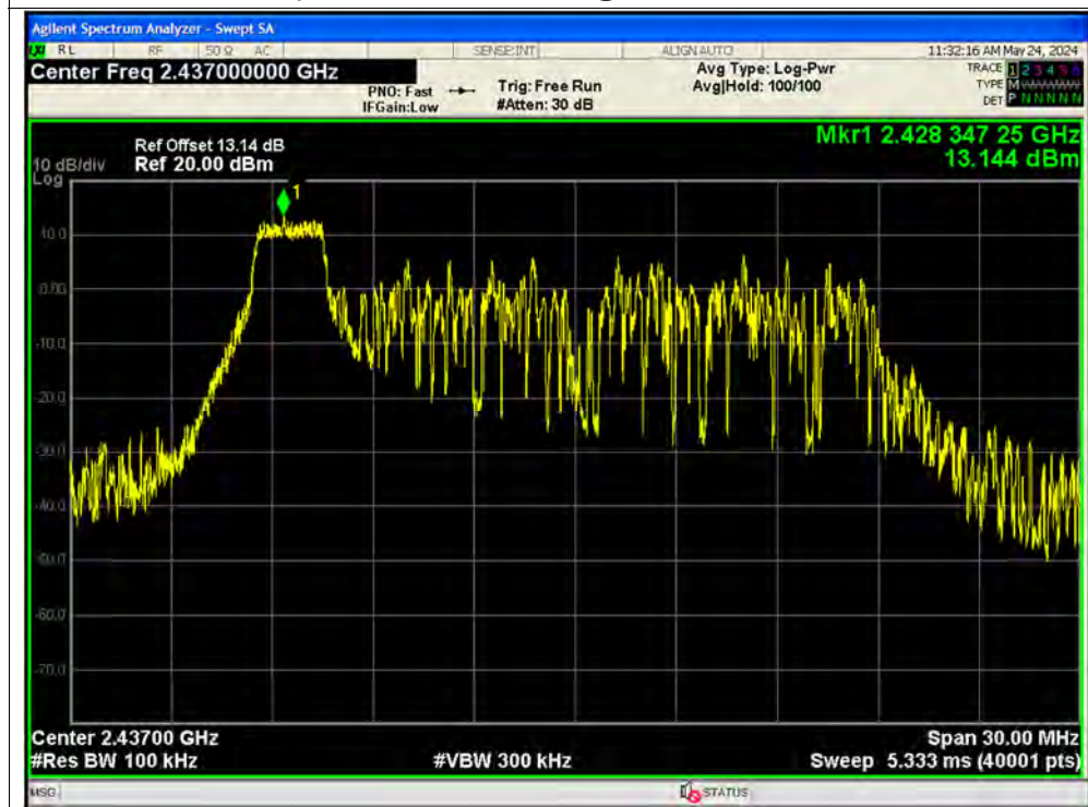
Tx. Spurious NVNT ax20 26@0 2437MHz Ant2 Emission
