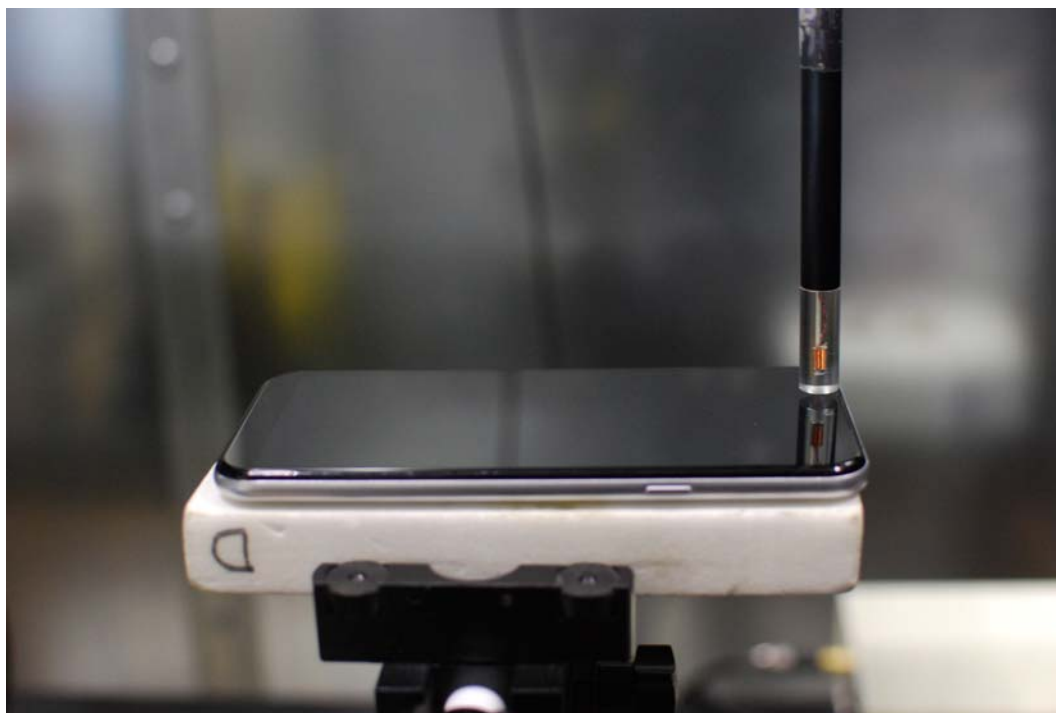
Figure 16-1 Test Setup for Wireless Device
