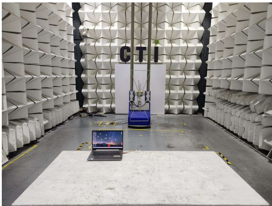
Radiated spurious emission Test Setup-1(Below 1GHz)
