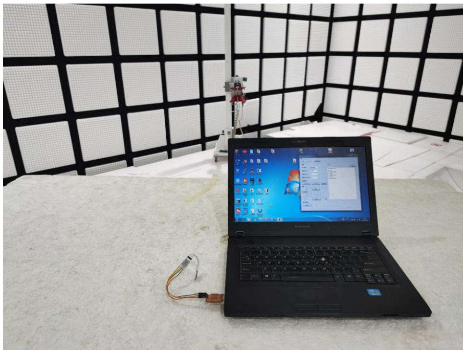
Radiated spurious emission Test Setup-3(Above 1GHz)
