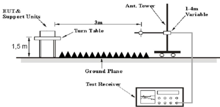
The radiated emission Below 1GHz tests were performed in the 3 meters chamber test site, above 1GHz tests were performed in the 3 meters chamber test site, using the setup accordance with the ANSI C63.10-2013. The specification used was the FCC 15.209, and FCC 15.247 limits.
