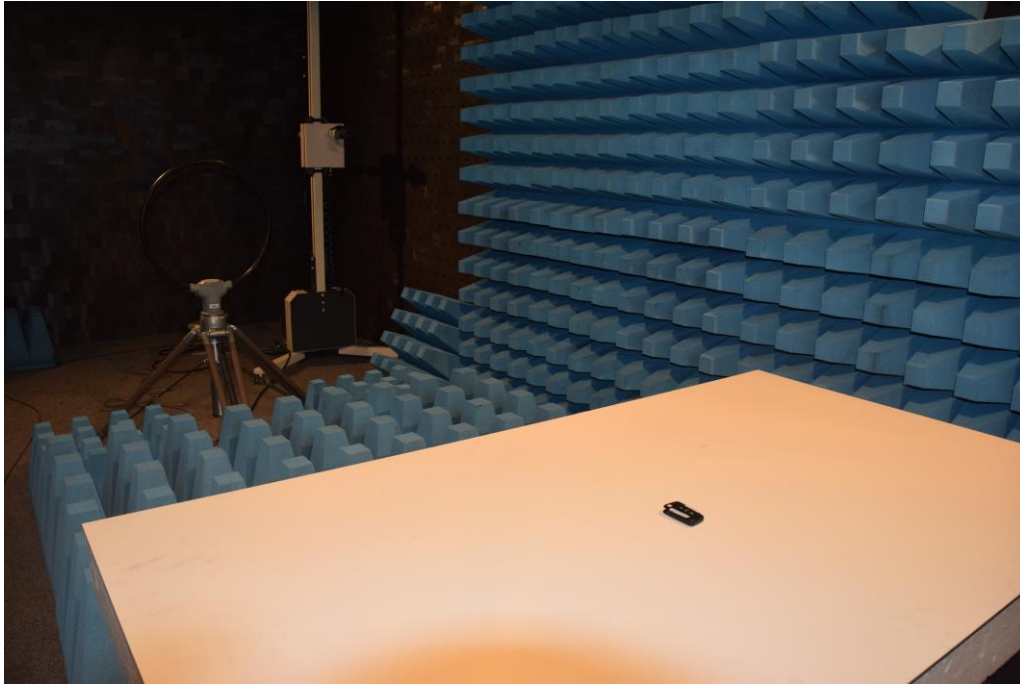
Picture 3: CDC, test setup radiated emission test 9 kHz -30 MHz of FS14T, version FS14TK (side view)
