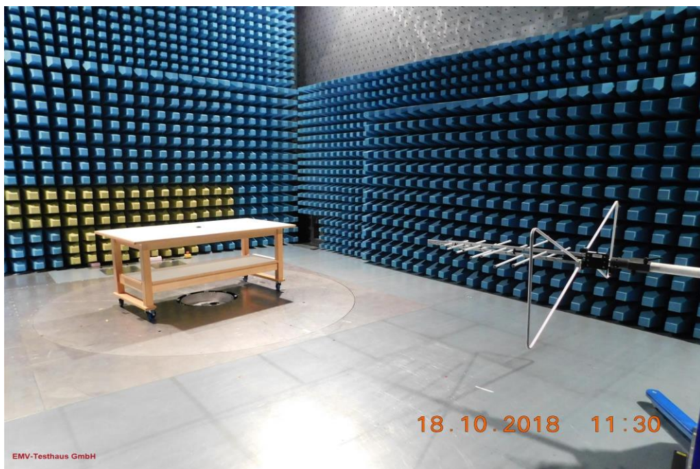
Picture 8: SAC, radiated emission test 30 MHz -1 GHz of FS14T, version FS14TK (rear view)
