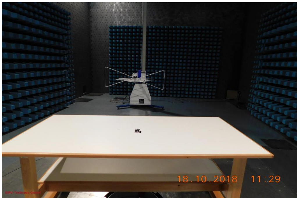
Picture 5: SAC, radiated emission test 30 MHz -1 GHz of FS14T, version FS14T (front view)
