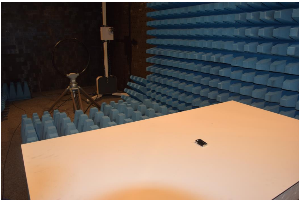
Picture 2: CDC, test setup radiated emission test 9 kHz -30 MHz of FS14T, version FS14T (side view)
