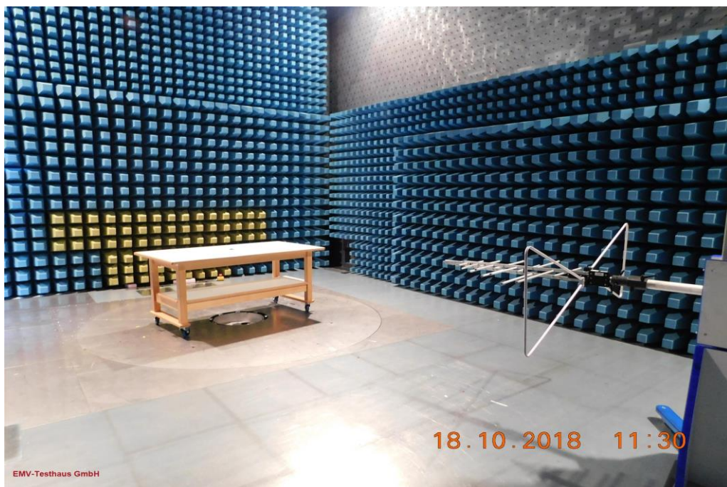
Picture 6: SAC, radiated emission test 30 MHz -1 GHz of FS14T, version FS14T (rear view)
