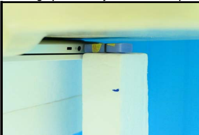
Horizontal Up of EUT Tested at 5 mm
