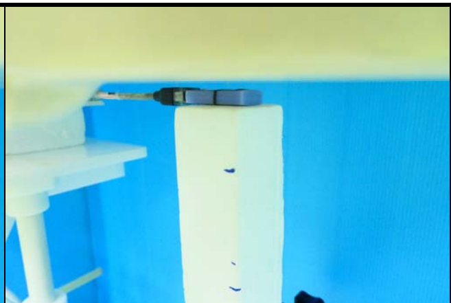
Horizontal Down of EUT Tested at 5 mm
