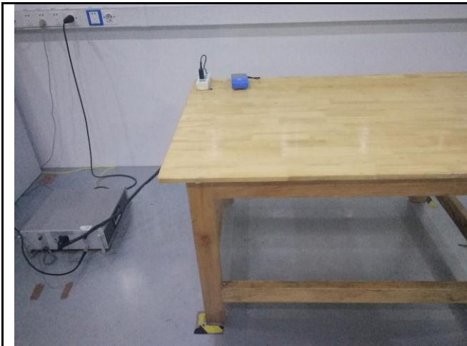
Conducted Emissions Test Setup Front View
