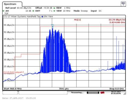
6.5.12. 960 MHz to 8 GHz Vertical at 1 Meter (Channel 4, 110 kbps, 64M PRF)
