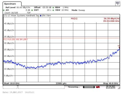
6.5.28. 18 to 40 GHz Vertical at 0.3 Meter (all modes of operation)
