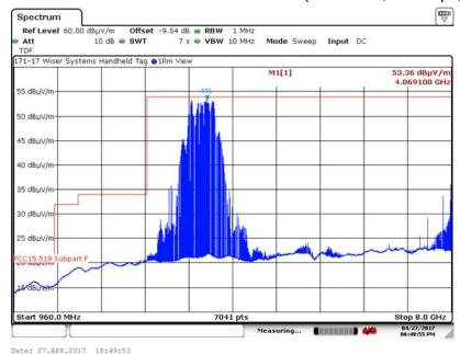
6.5.8. 960 MHz to 8 GHz Vertical at 1 Meter (Channel 2, 6.8 Mbps, 64M PRF)
