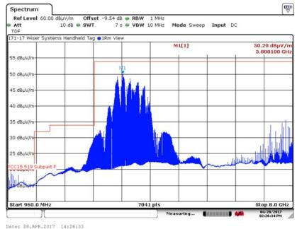
6.5.14. 960 MHz to 8 GHz Vertical at 1 Meter (Channel 4, 6.8 Mbps, 16M PRF)
