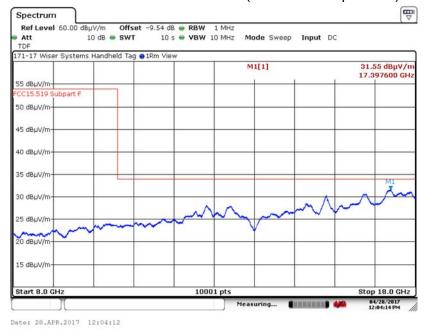
6.5.26. 8 to 18 GHz Vertical at 1 Meter (all modes of operation)
