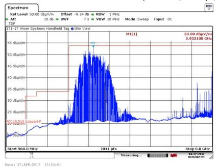
6.5.10. 960 MHz to 8 GHz Vertical at 1 Meter (Channel 4, 110 kbps, 16M PRF)
