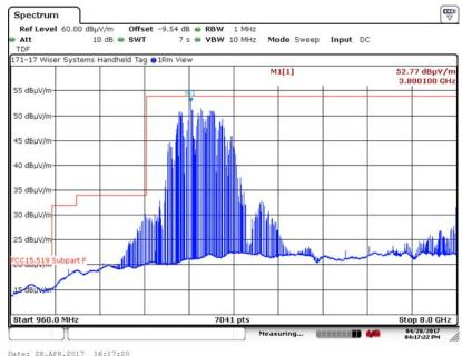
6.5.16. 960 MHz to 8 GHz Vertical at 1 Meter (Channel 4, 6.8 Mbps, 64M PRF)
