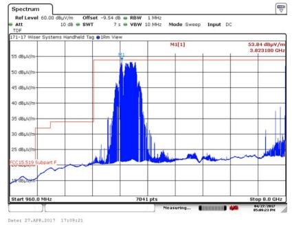
6.5.4. 960 MHz to 8 GHz Vertical at 1 Meter (Channel 2, 110 kbps, 64M PRF)
