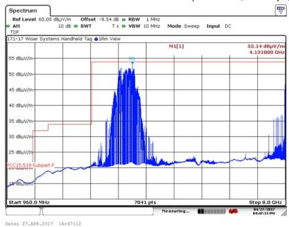
6.5.2. 960 MHz to 8 GHz Vertical at 1 Meter (Channel 2, 110 kbps, 16M PRF)
