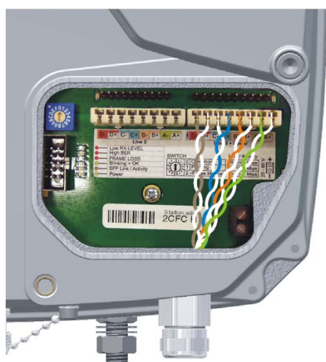
Figure 20 Finished assembly of the connection cable Cat7 S-STP
