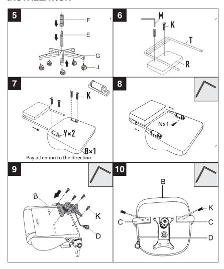
**Note:** All screws havebeenpreassembled to the accessories Please remove them from the accessories before assembling
