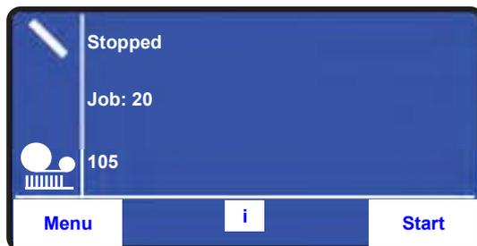
This will put the printer into 'Stopped' mode and the printer will ignore 'Print Go' signals.
