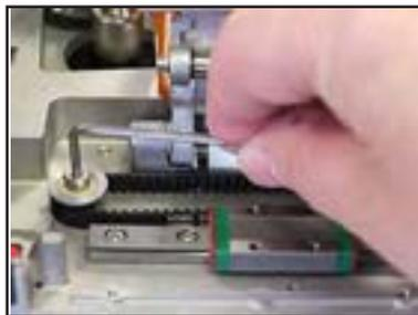
Replace the belt pulley and secure
