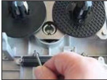
Remove the two retaining screws from the ribbon tension spring cover.
