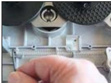
Unscrew the spring retaining screw.
