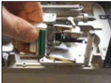
Remove the printhead from the print module.
