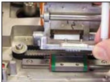
Remove the carriage plate from the linear bearing slide.
