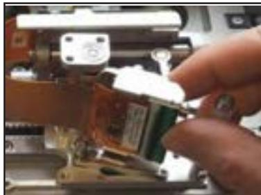
Push the printhead away from the peel roller.
