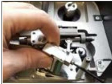
Push the printhead forward and turn the securing screw through 90° clockwise
