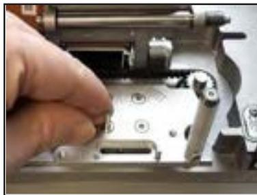
Remove the four retaining screws from the print module carriage plate
