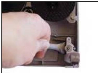
Fit a new tension roller assembly and secure.
