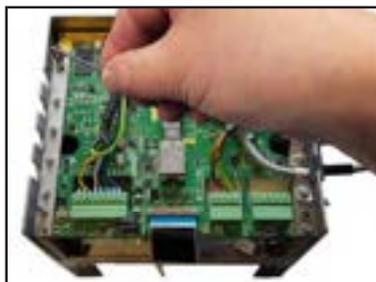
Use a 2.5mm hex key to remove the cable clamp plate screws.
