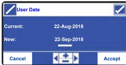
Use the quad buttons to change the user date and press the 'Accept' button to confirm.
