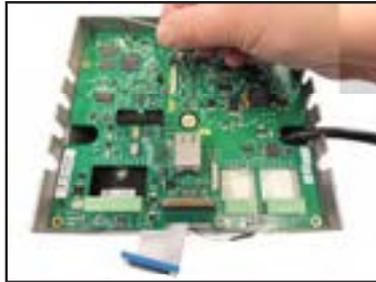
Remove the two remaining screws from the PCB.
