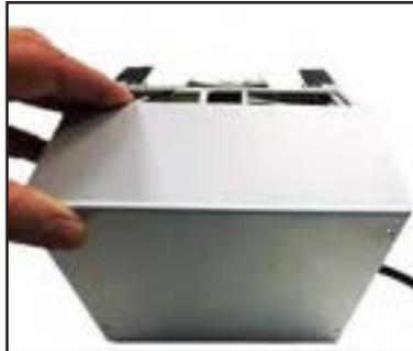
Undo the four retaining screws and remove the cover from the printer body
