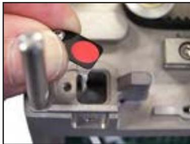
Remove the sensor from the printer body.
