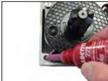
Apply Loctite 222 to the replacement movement roller assembly screw hole before fitting the replacement roller
