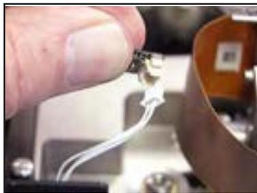
Disconnect the sensor from the wire connector.
