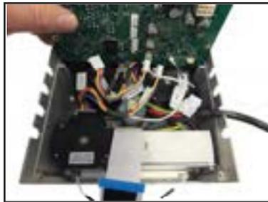
Disconnect all connectors and remove the PCB.
