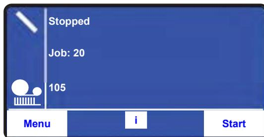
Press the 'Start' button to switch the printer into 'Producing'. Any fault condition present will stop the printer entering 'Producing' mode. See page 153 , 'Faults and Warning Messages'.
