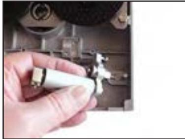
Remove the tension roller assembly from the cassette.
