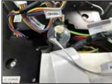
Remove the printer PCB and locate the solenoid
