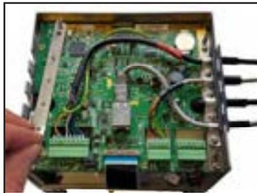
Remove the cable clamp plate from the printer.
