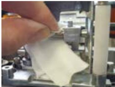
Use a printhead wipe to clean off any debris from the gimble pin
