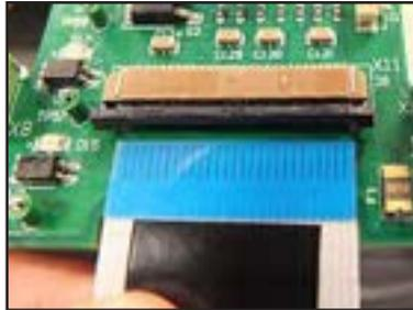
Remove the printhead ribbon from the connector.
