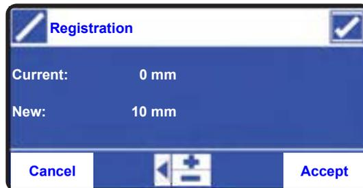
Use the + and - buttons to increase or decrease the units, or alternatively enter the required value using the numerical keypad
