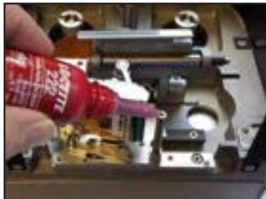
Apply Loctite 222 to the replacement peel roller assembly screw hole, wiping away any excess before fitting the peel roller
