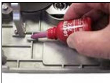
Add Loctite 222 to the spring retaining screw hole.
