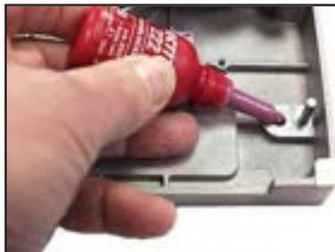
Before fitting a replacement assembly add Loctite 222 to the screw hole.
