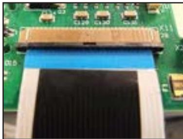
Locate the printhead ribbon PCB connector
