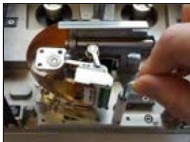
After securing, rotate the roller to ensure it is moving freely
