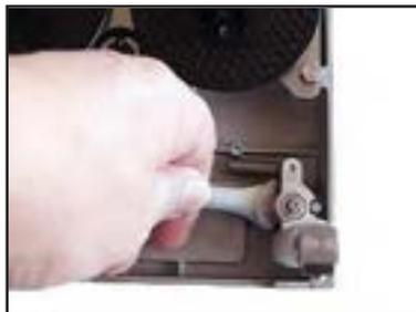
Use a 10mm wrench to unscrew the tension roller assembly from the cassette.
