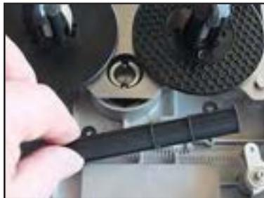
Remove the tension spring cover and place to the side.
