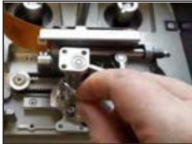
Remove the two retaining screws from the print module
