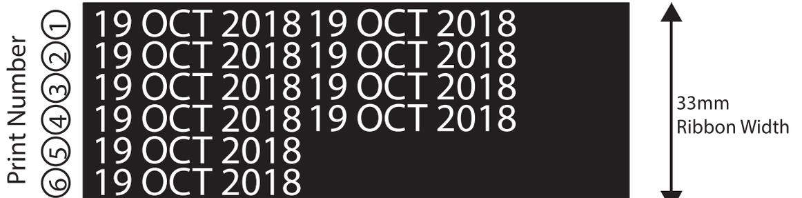
As the relative position of the print will move on the substrate. This mode is useful if the final position of the text on the substrate is not important.
