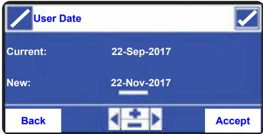
Use the keypad to edit the date. Move the cursor along the line to edit each field. User dates do not rollover automatically and will remain until a new job is selected or the current job is reselected.
