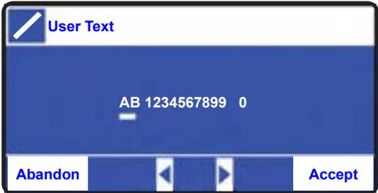
Use the keypad to add or edit the text. Move the cursor along the line of text to edit each character. User text is limited to 16 characters, including spaces and is alphanumeric.
