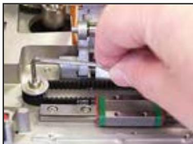
Use a 2.5mm hex key to remove the belt pulley
