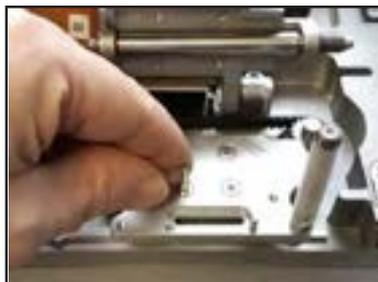
Replace the printhead carriage and secure
