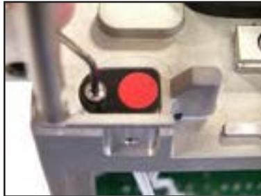
Use a 1.5mm hex key to remove the sensor retaining screw.
