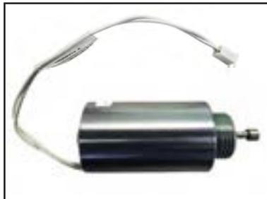
The solenoid is screwed directly into the printer body. When fitting a replacement, use Loctite 222 to secure the solenoid to the printer body
