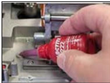
Add Loctite 222 to the belt pulley screw hole
