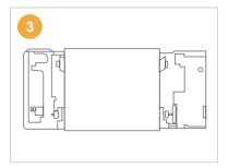
Insert the fan-fold label or roll label from outside, adjust the paper guide to fit the width of paper
