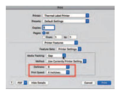
Tips: For the darkness, large number means higher darkness, if labels print out light, you can adjust it to large value, 8-14 is recommended.
