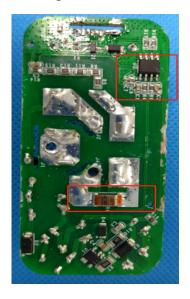
S40TPB is different from S40TPB Lite in that there is an electric quantity measurement and detection circuit, the rest are the same
