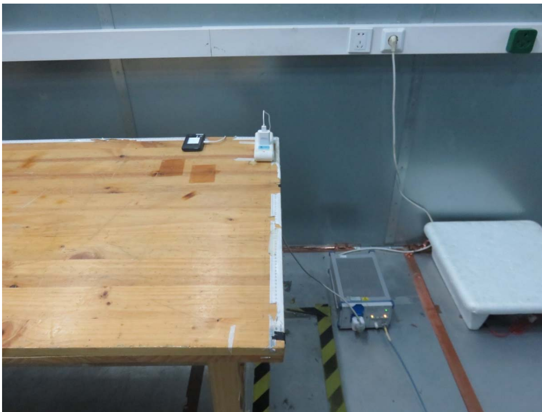
Picture 2 Conducted Emission Test Setup
