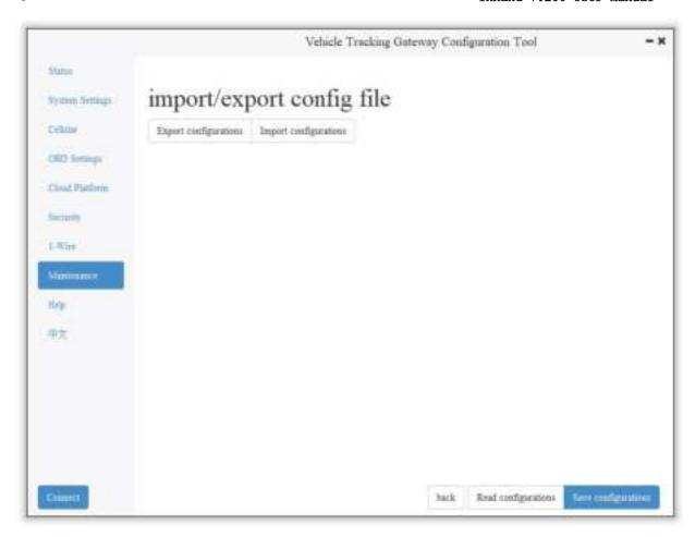
To back up configuration, click "Export configuration". The configuration tool can read device configuration and pop up file storage window. Enter the name of the backup file, and click "Open".
