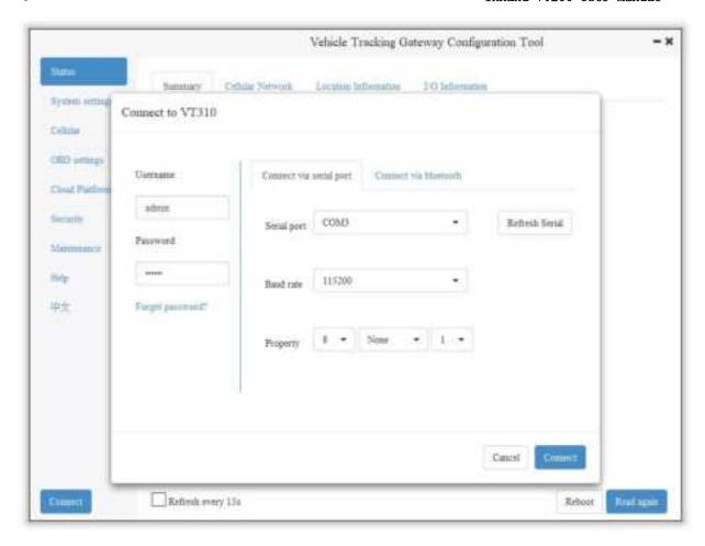
You can also use computer Bluetooth (4.2 or above) to connect the device. Click "Connect device", enter the user name and password (default: admin/123456), select the Bluetooth device with the same name as the device SN (SN can be found on the device nameplate), and click Connect ", as is shown below.
