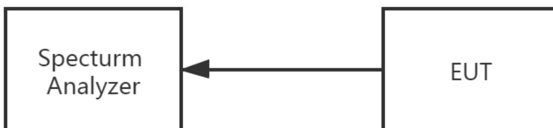
The EUT which is powered by the battery, is connected to the Spectrum Analyzer; the RF load attached to the EUT antenna terminal is 50 Ohm; the path loss as the factor is calibrated to correct the reading. Make the measurement with the spectrum analyzer's resolution bandwidth(RBW) = 100 kHz. In order to make an accurate measurement, set the span greater than RBW.
