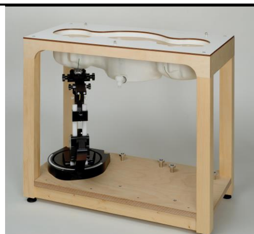
Fig. 8.7 Photo of SAM Twin Phantom
