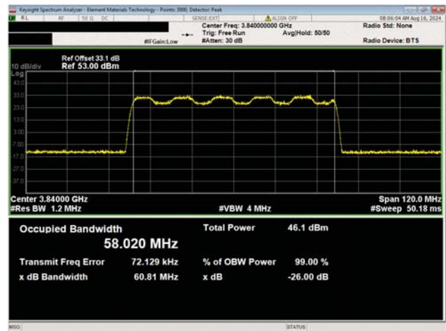
Port 1 60 MHz Channel Bandwidth 16QAM Modulation Mid Channel, 3840.00 MHz
