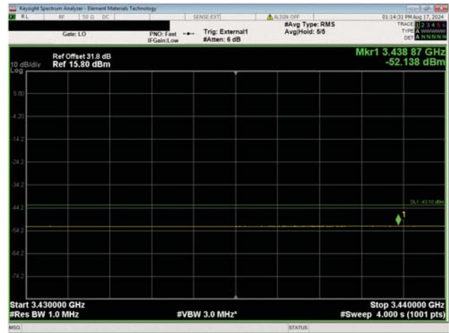
Port 1 10 MHz Channel Bandwidth QPSK Modulation Low Channel, 3455.01 MHz
