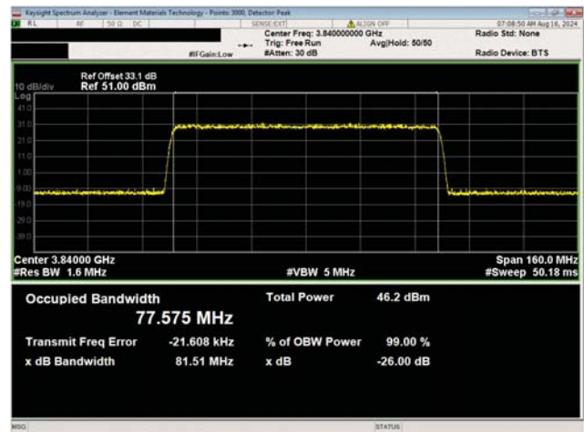
Port 1 80 MHz Channel Bandwidth 256QAM Modulation Mid Channel, 3840.00 MHz
