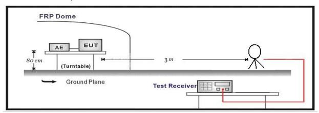
Below 1GHz Test Setup:
