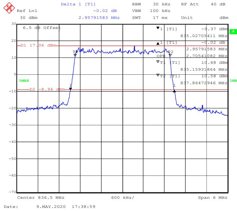
**16-QAM (5.0 MHz) - 99% Occupied & 26 dB Emissions Bandwidth, Middle channel**
