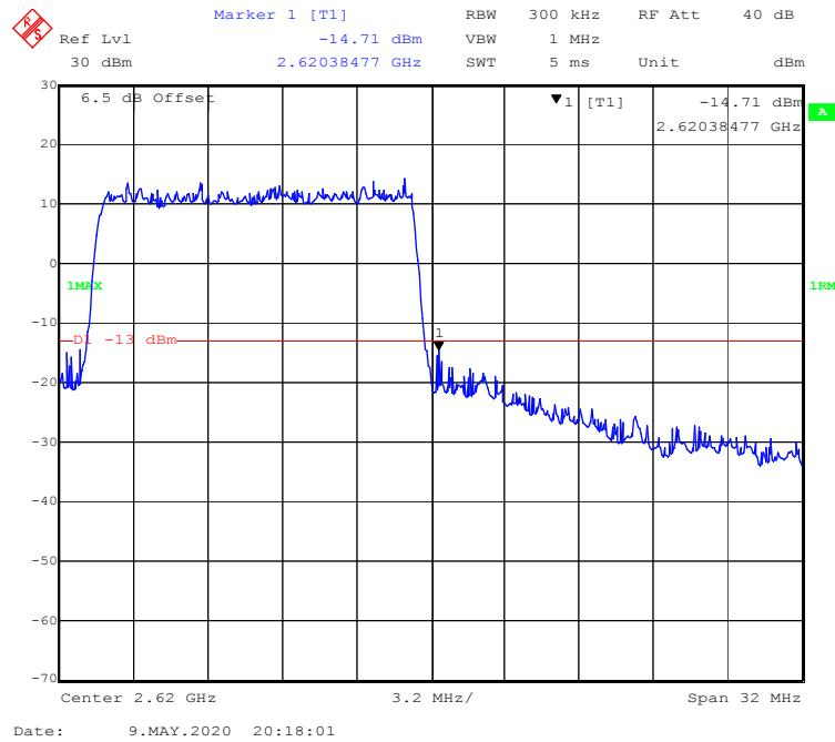
**QPSK (20.0 MHz, FULL RB) - Left Band Edge**
