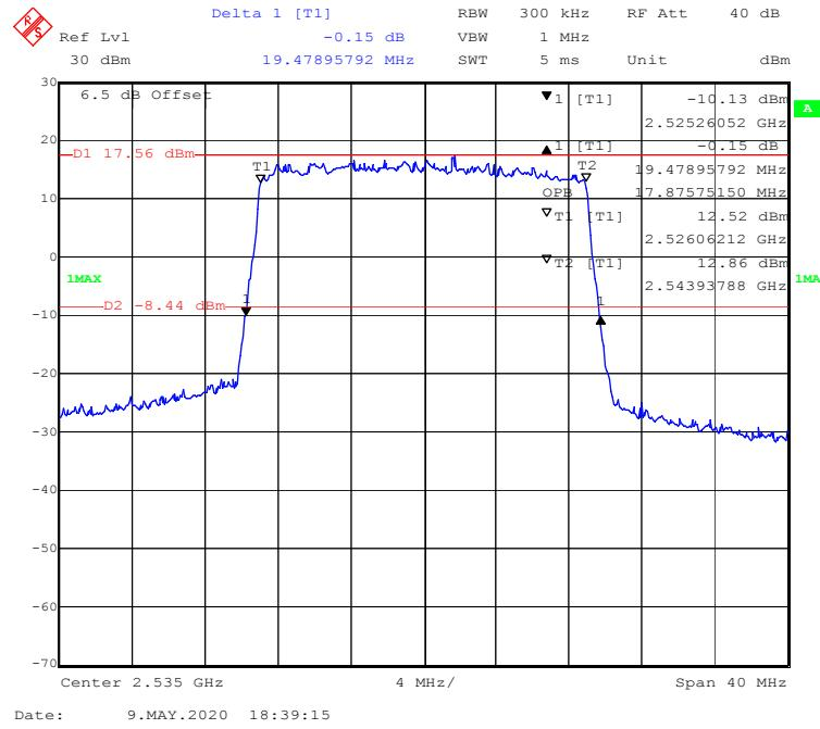
**16-QAM (5.0 MHz) - 99% Occupied & 26 dB Emissions Bandwidth, Middle channel**
