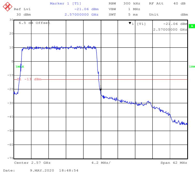
**16-QAM (5.0 MHz, FULL RB) - Left Band Edge**
