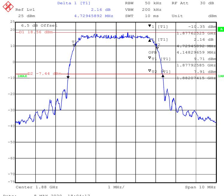
**99% Occupied & 26 dB Emissions Bandwidth for WCDMA (HSUPA) Mode**
