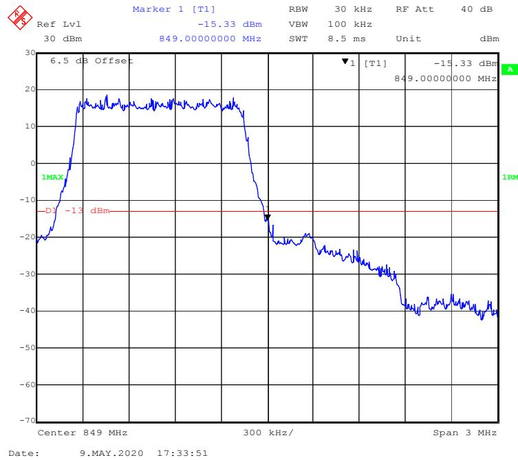
**16-QAM (3.0 MHz, FULL RB) - Left Band Edge**
