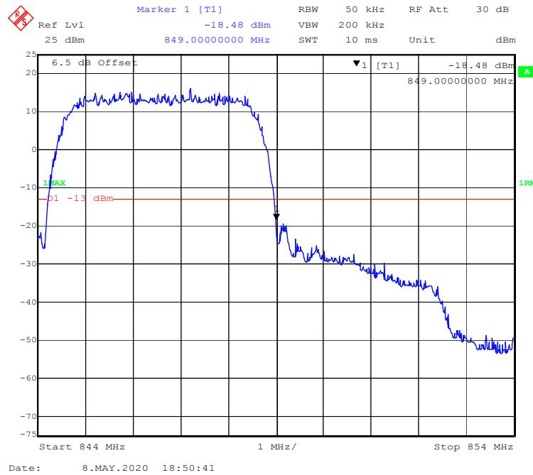
**PCS 1900 Band:****GPRS Mode, Left Band Edge**
