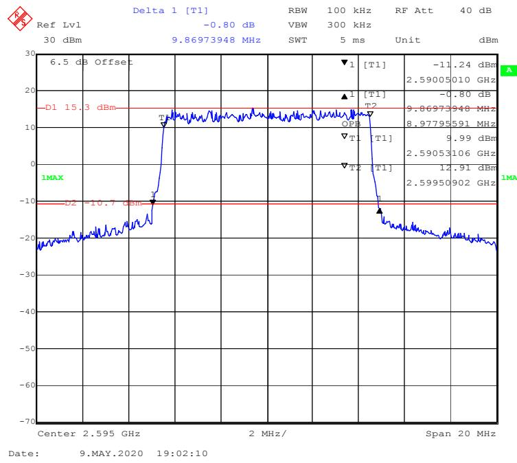
**16-QAM (15.0 MHz) - 99% Occupied & 26 dB Emissions Bandwidth, Middle channel**
