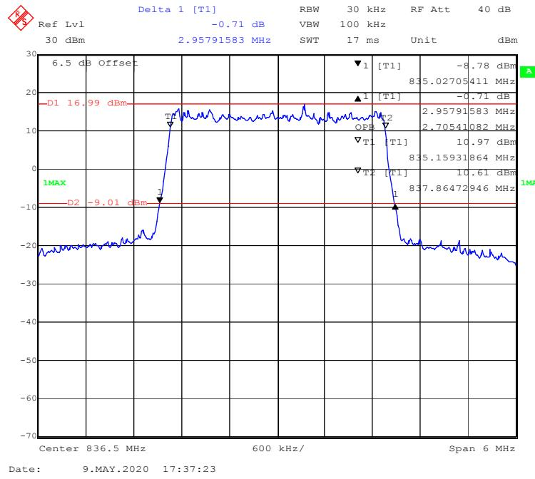
**QPSK (5.0MHz) - 99% Occupied & 26 dB Emissions Bandwidth, Middle channel**
