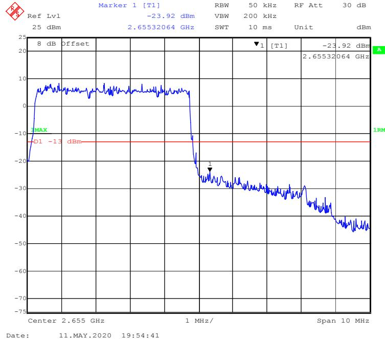
**QPSK (10.0 MHz, FULL RB) - Left Band Edge**
