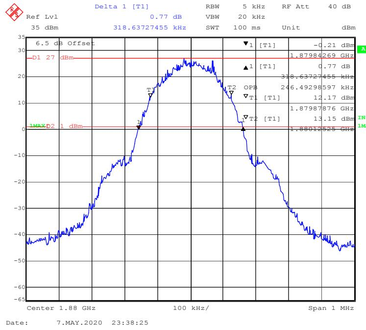
**99% Occupied & 26 dB Emissions Bandwidth for EGPRS (8PSK) Mode**
