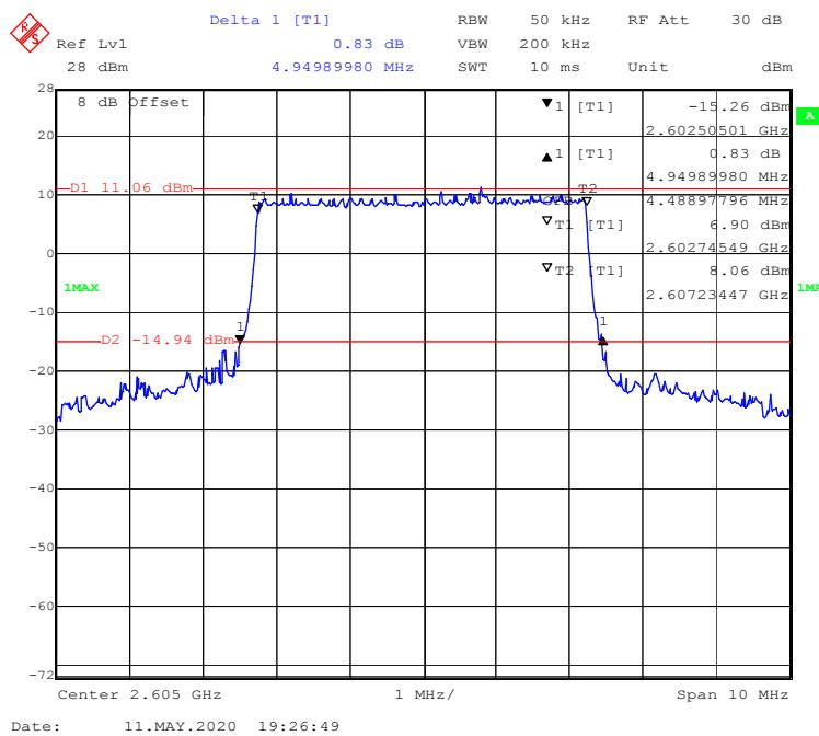
**QPSK (10.0 MHz) - 99% Occupied & 26 dB Emissions Bandwidth, Middle channel**
