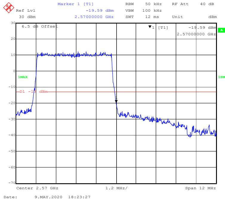
**16-QAM (10.0 MHz, FULL RB) - Left Band Edge**
