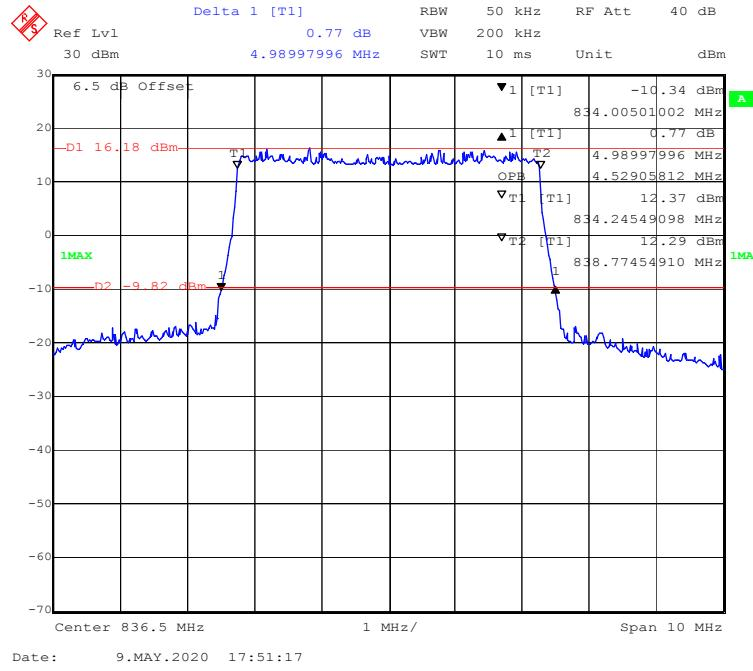
**16-QAM (10.0 MHz) - 99% Occupied & 26 dB Emissions Bandwidth, Middle channel**
