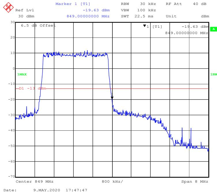
**16-QAM (5.0 MHz, FULL RB) - Left Band Edge**
