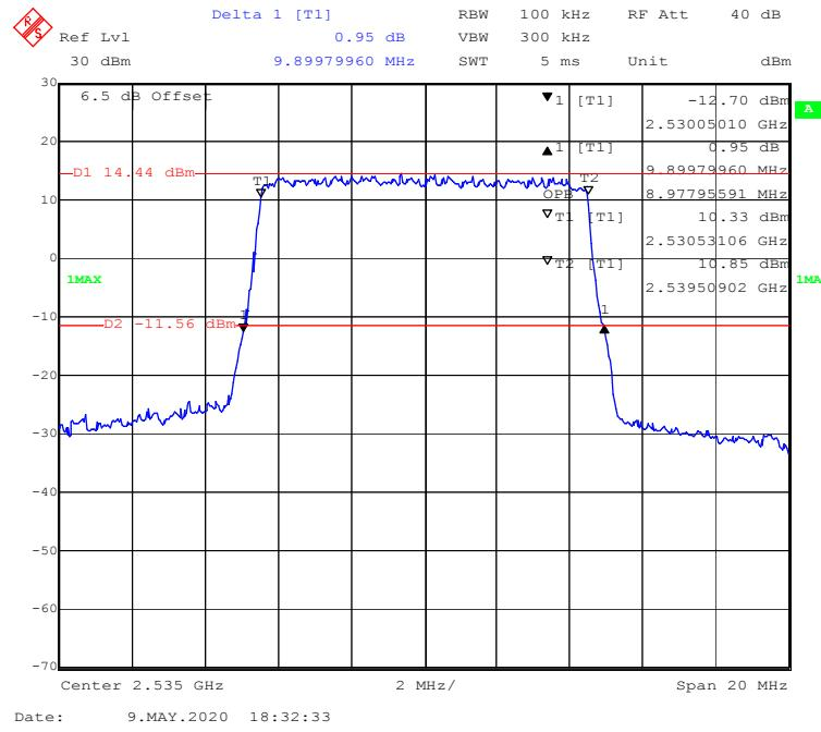
**QPSK (15.0MHz) - 99% Occupied & 26 dB Emissions Bandwidth, Middle channel**
