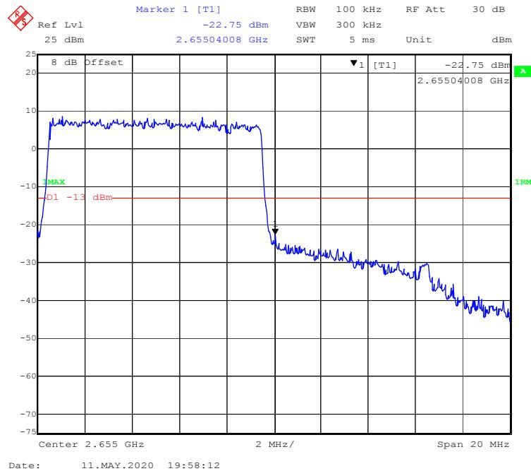
**QPSK (15.0 MHz, FULL RB) - Left Band Edge**
