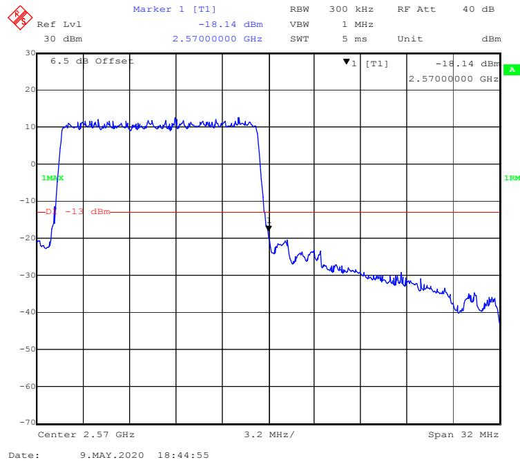
**16-QAM (20.0 MHz, FULL RB) - Left Band Edge**
