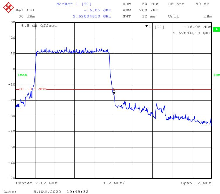
**16-QAM (10.0 MHz, FULL RB) - Left Band Edge**
