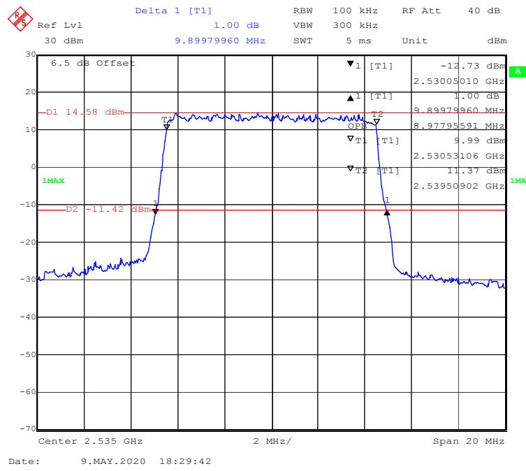
**16-QAM (15.0 MHz) - 99% Occupied & 26 dB Emissions Bandwidth, Middle channel**
