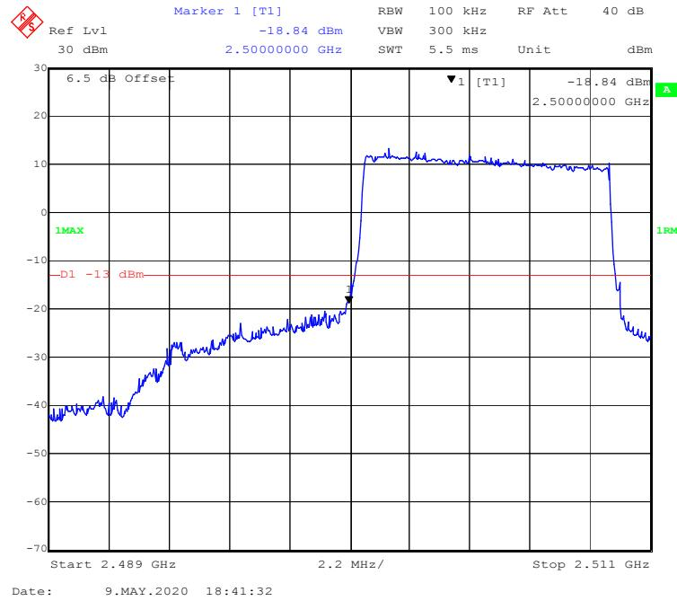
**16-QAM (10.0 MHz, FULL RB) - Right Band Edge**
