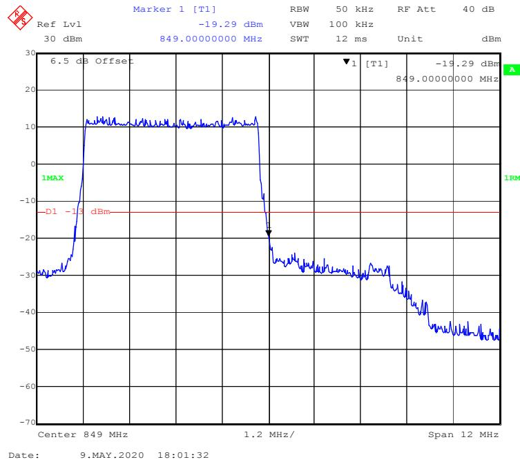
**16-QAM (10.0 MHz, FULL RB) - Left Band Edge**
