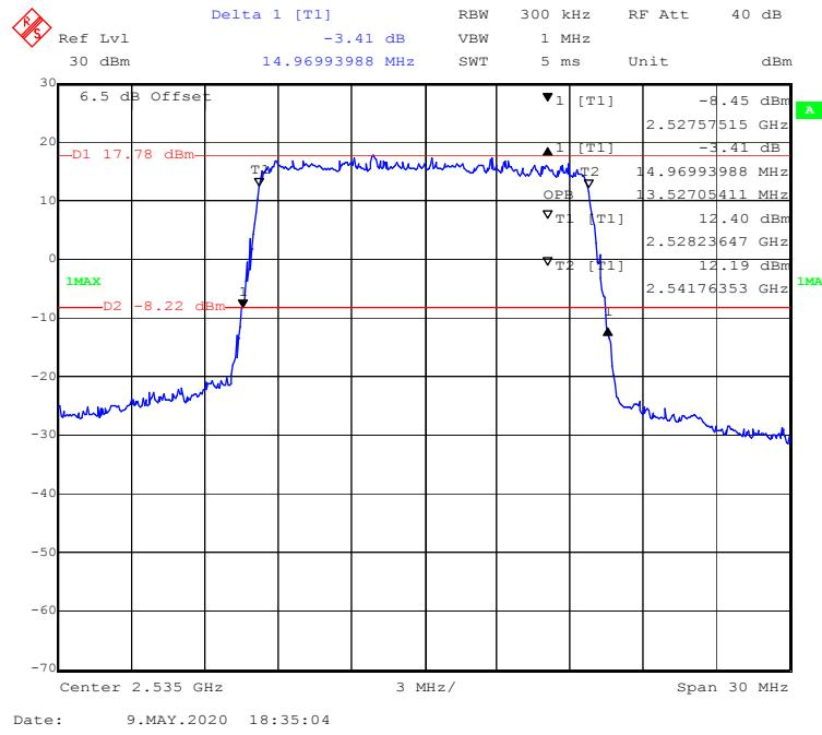
**16-QAM (20.0 MHz) - 99% Occupied & 26 dB Emissions Bandwidth, Middle channel**
