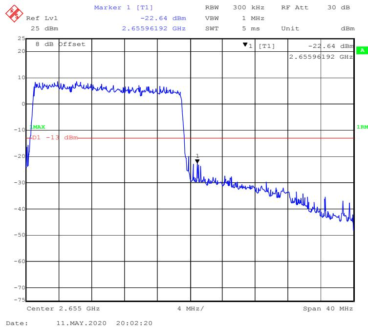
**16-QAM (5.0 MHz, FULL RB) - Left Band Edge**
