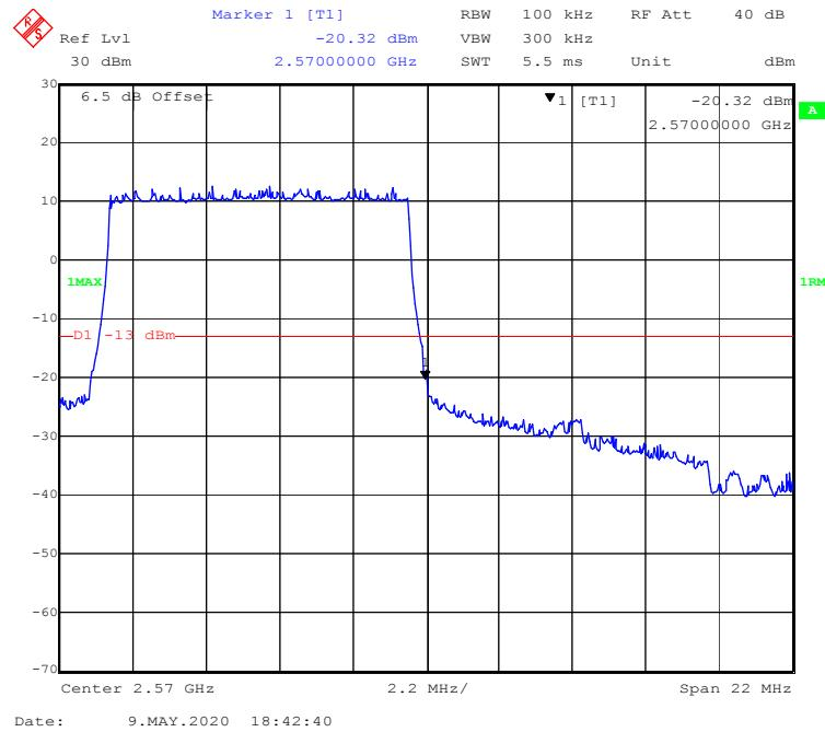
**16-QAM (15.0 MHz, FULL RB) - Left Band Edge**
