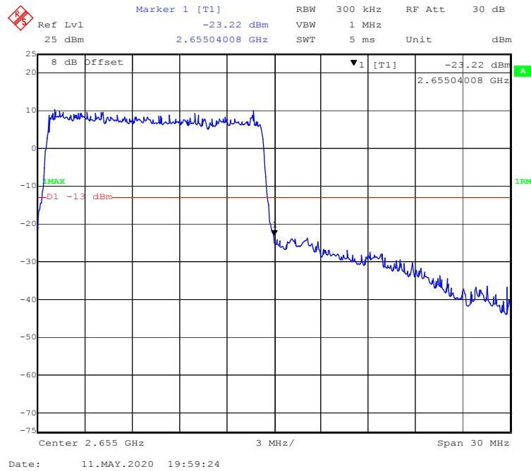
**16-QAM (20.0 MHz, FULL RB) - Left Band Edge**
