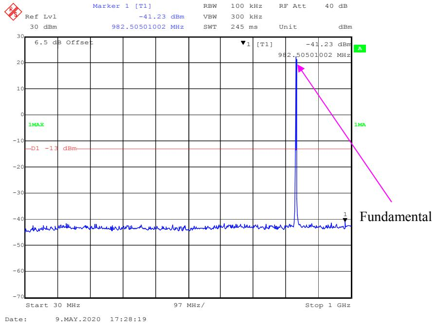
**1 GHz – 10 GHz (QPSK, 1.4 MHz, Middle Channel)**
