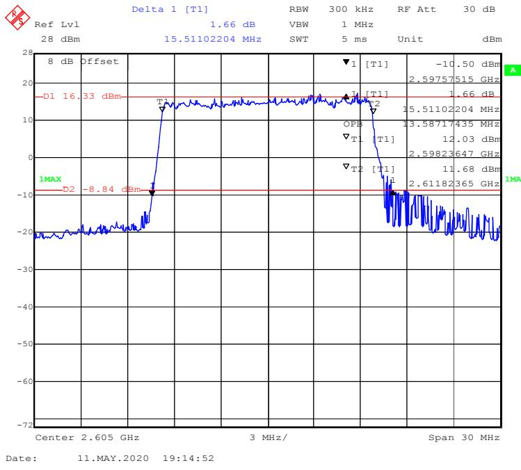
**16-QAM (20.0 MHz) - 99% Occupied & 26 dB Emissions Bandwidth, Middle channel**
