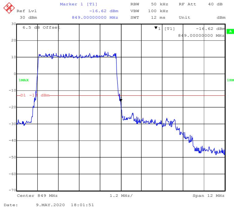
**QPSK (10.0 MHz, FULL RB) - Left Band Edge**
