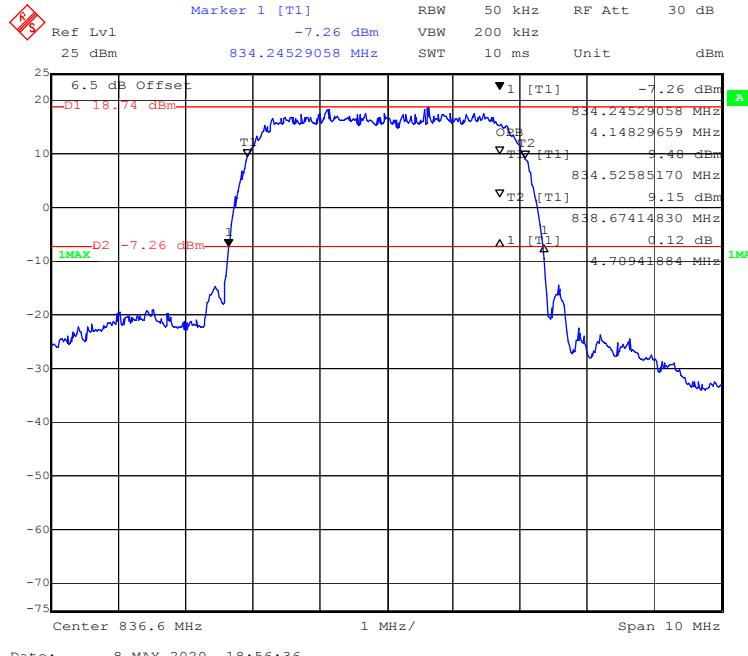
**99% Occupied & 26 dB Emissions Bandwidth for WCDMA (HSUPA) Mode**
