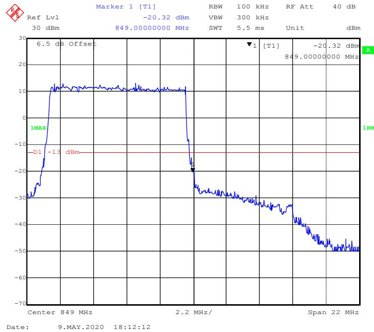
**LTE Band 7:****QPSK (5.0 MHz, FULL RB) - Left Band Edge**
