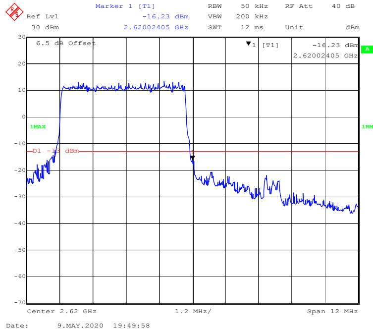
**QPSK (10.0 MHz, FULL RB) - Left Band Edge**
