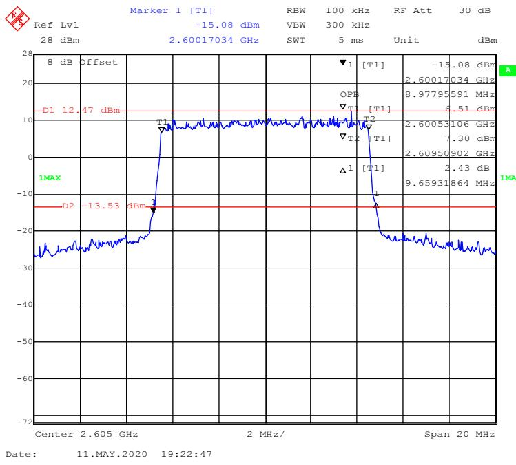
**16-QAM (15.0 MHz) - 99% Occupied & 26 dB Emissions Bandwidth, Middle channel**
