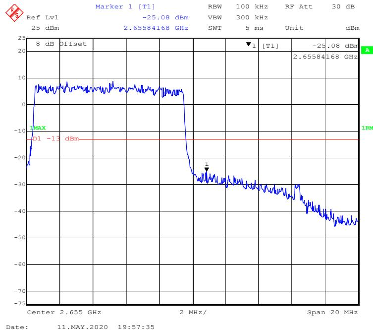
**16-QAM (15.0 MHz, FULL RB) - Left Band Edge**
