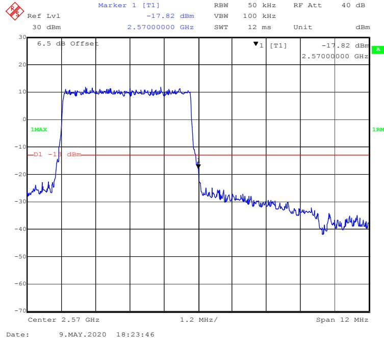
**QPSK (10.0 MHz, FULL RB) - Left Band Edge**
