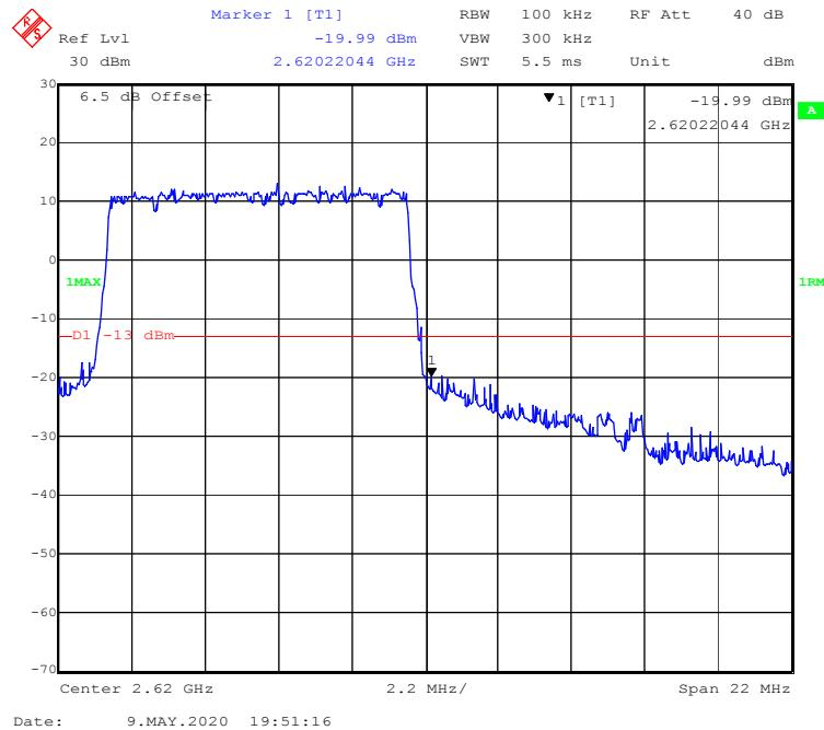
**QPSK (15.0 MHz, FULL RB) - Left Band Edge**
