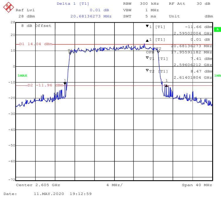
**16-QAM (5.0 MHz) - 99% Occupied & 26 dB Emissions Bandwidth, Middle channel**
