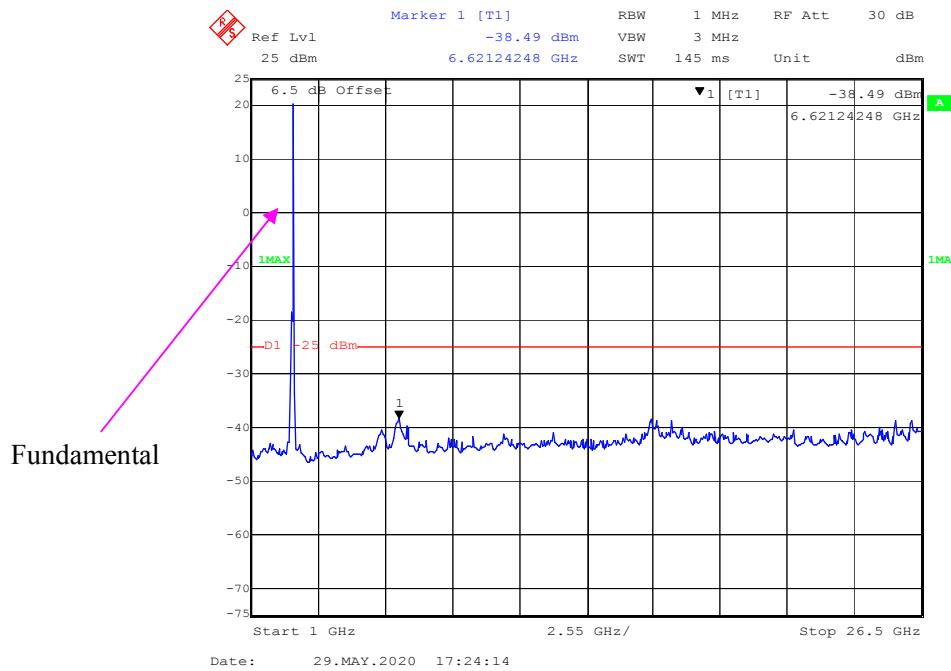
**30 MHz - 1 GHz (16QAM, 20.0 MHz, Middle Channel)**
