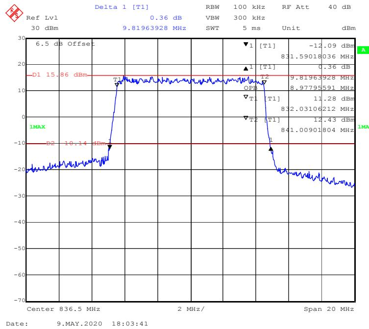
**16-QAM (1.4 MHz) - 99% Occupied & 26 dB Emissions Bandwidth, Middle channel**
