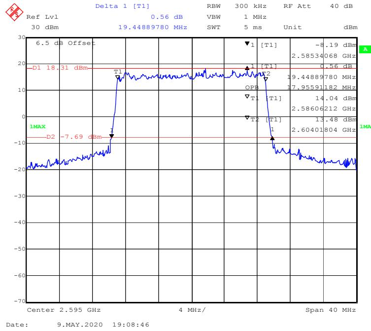
**16-QAM (5.0 MHz) - 99% Occupied & 26 dB Emissions Bandwidth, Middle channel**
