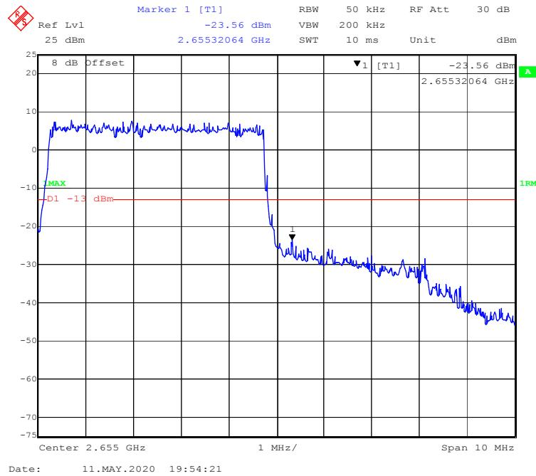
**16-QAM (10.0 MHz, FULL RB) - Left Band Edge**
