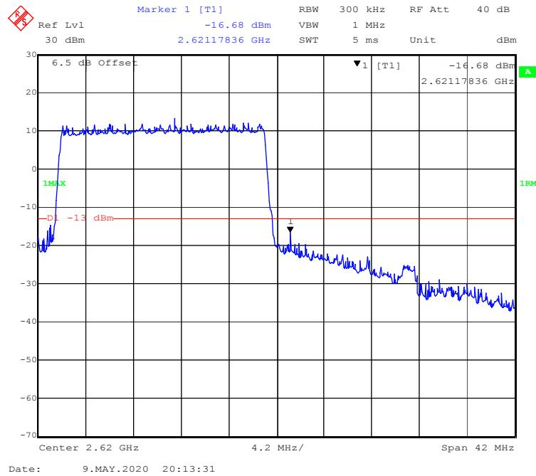
**16-QAM (5.0 MHz, FULL RB) - Left Band Edge**
