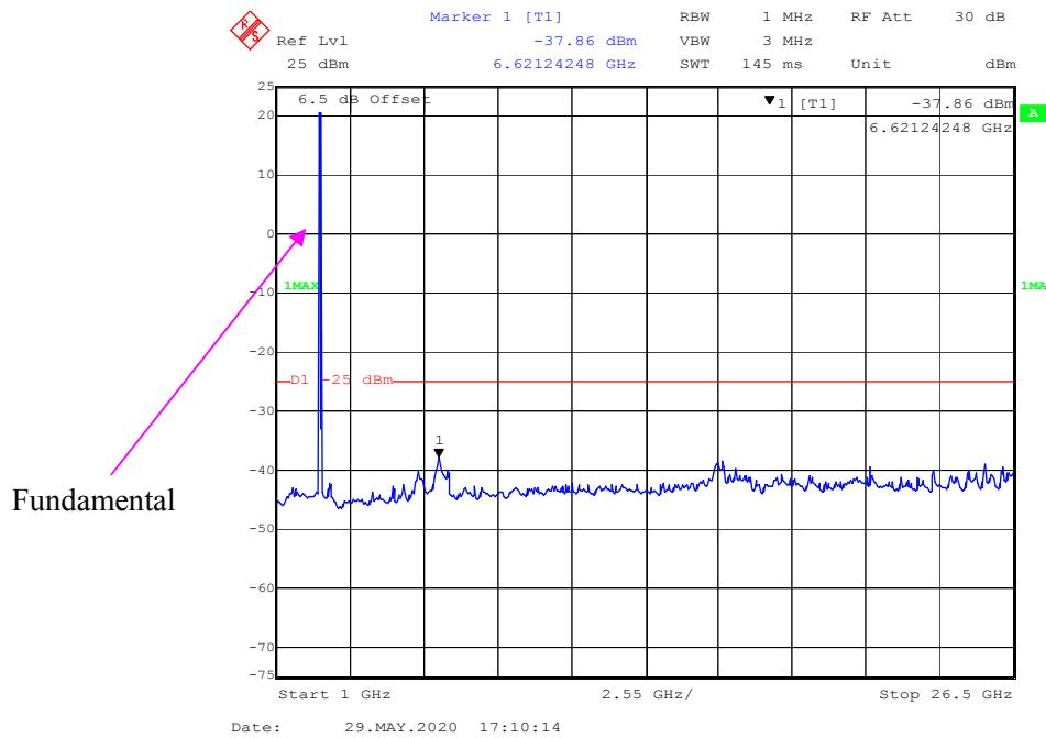
**30 MHz - 1 GHz (16QAM, 20.0 MHz, Middle Channel)**
