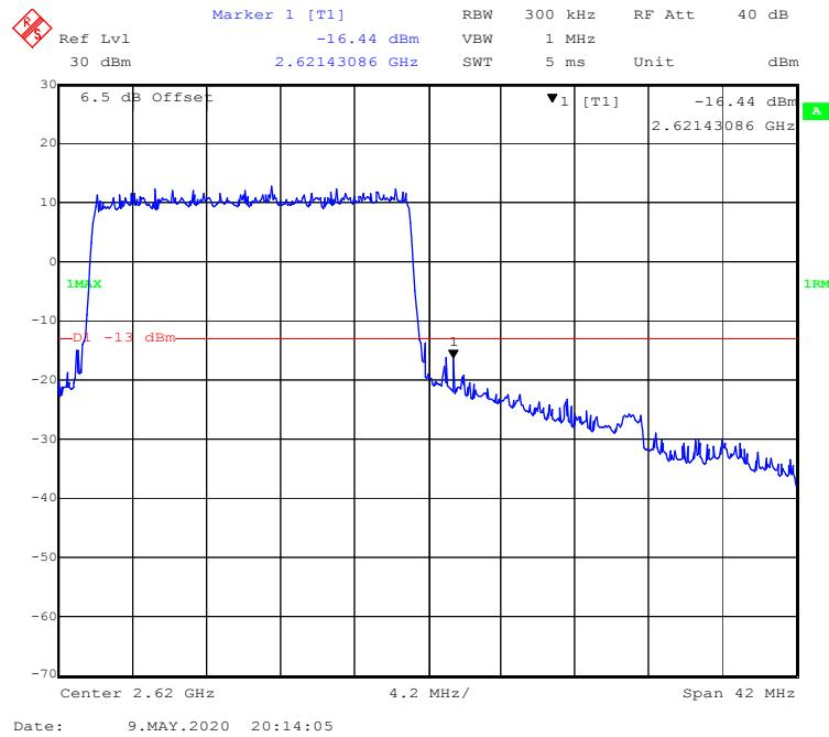
**LTE Band 41:****QPSK (5.0 MHz, FULL RB) - Left Band Edge**
