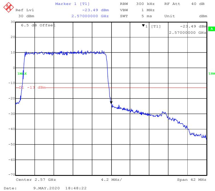
**LTE Band 38:****QPSK (5.0 MHz, FULL RB) - Left Band Edge**
