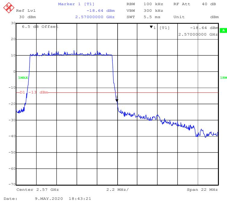
**QPSK (15.0 MHz, FULL RB) - Left Band Edge**
