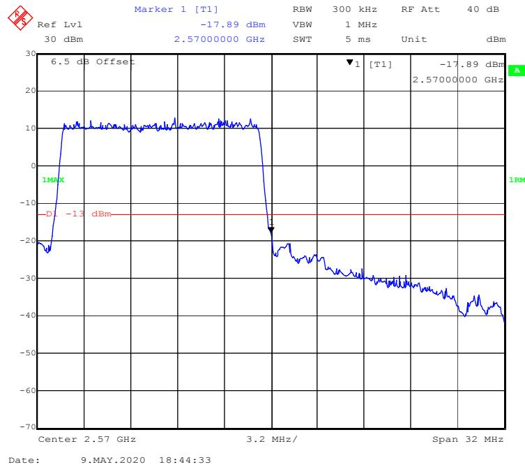
**QPSK (20.0 MHz, FULL RB) - Left Band Edge**
