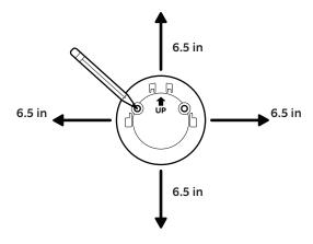
2. Install the mounting plate with the UP arrow pointing up. / Install the mounting plate with the UP arrow pointing up. / Install the mounting plate with the UP arrow pointing up.
