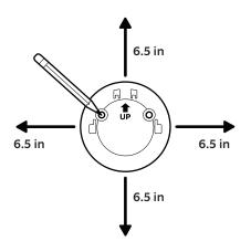
2. Install the mounting plate with the UP arrow pointing opposite of your desired viewing direction. / Install the mounting plate with the UP arrow pointing opposite of your desired viewing direction. / Install the mounting plate with the UP arrow pointing opposite of your desired viewing direction.
