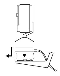
5. Secure your camera and bracket to the mounting plate by sliding until you feel a click. / Secure your camera and bracket to the mounting plate by sliding until you feel a click. / Secure your camera and bracket to the mounting plate by sliding until you feel a click.
