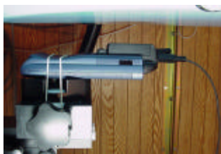
EUT with Visor Prism & 2.5cm separation distance
