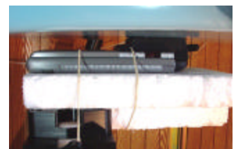
EUT with Visor Platinum Back touching phantom surface
