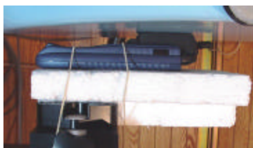
EUT with Visor Prism Back touching phantom surface
