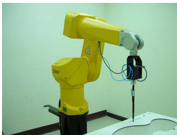
Fig. 5.2 Probe setup on robot
