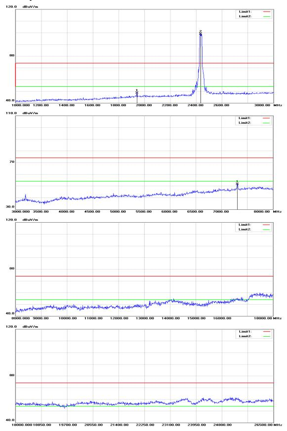
Operation Mode: TX / IEEE 802.11n HT 20 MHz / 2437 MHz Test Date: January 10, 2016
