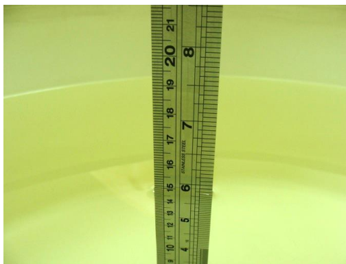
Fig 6.1 Photo of Liquid Height for Body SAR
