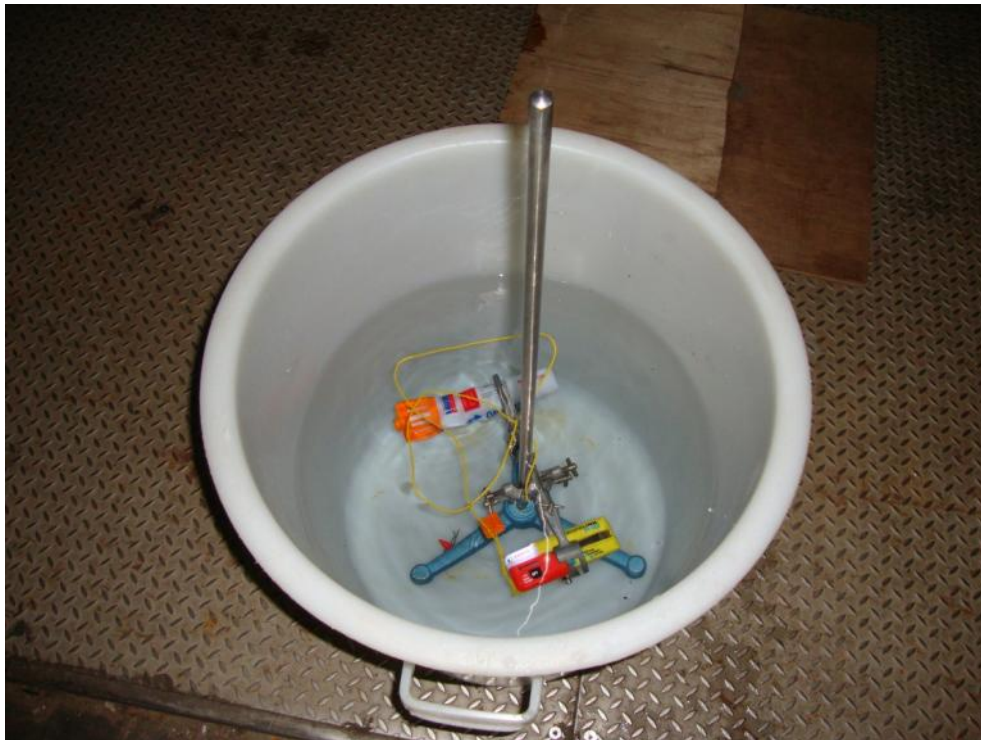
Test Set-up – Thermal Shock (submerged EUTs)
