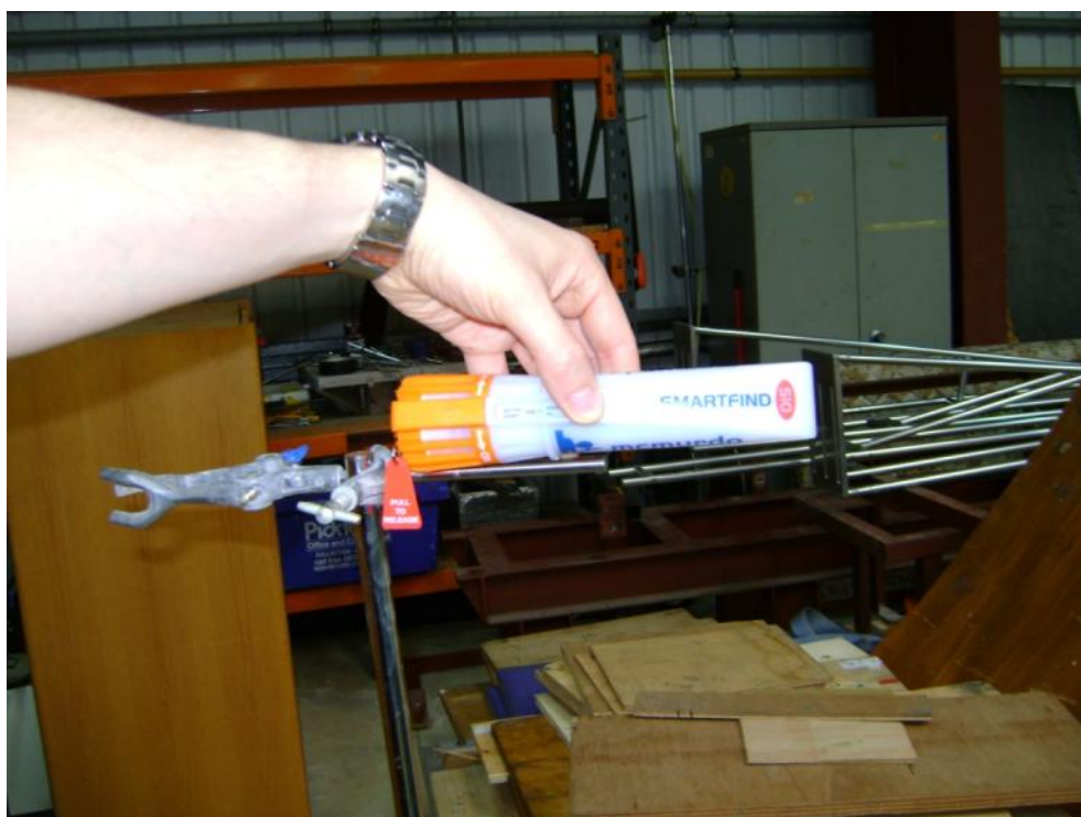
Test Set-up – Drop onto Hard Surface (Z502)
