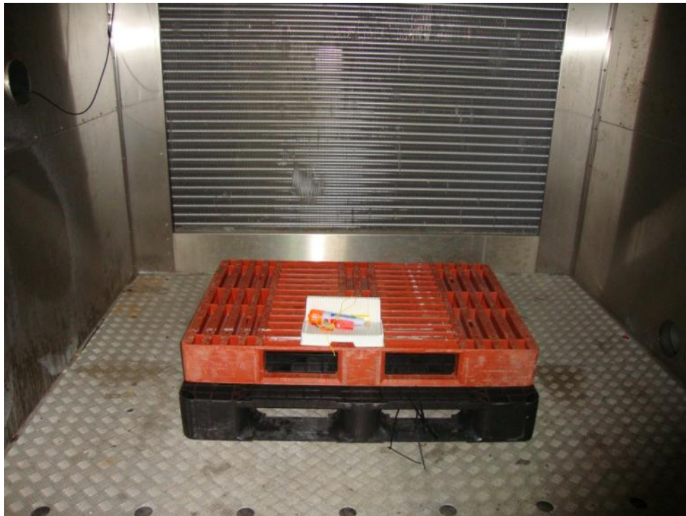
Test Set-up – Thermal Shock (EUT pre-conditioning)
