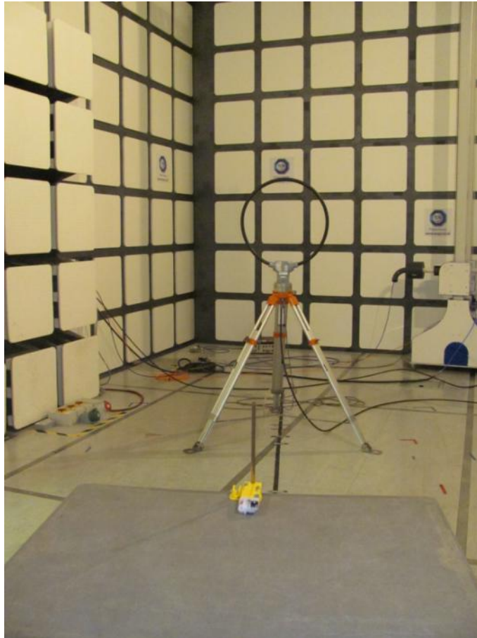
Test Set-up – Z501 Magnetic Emissions
