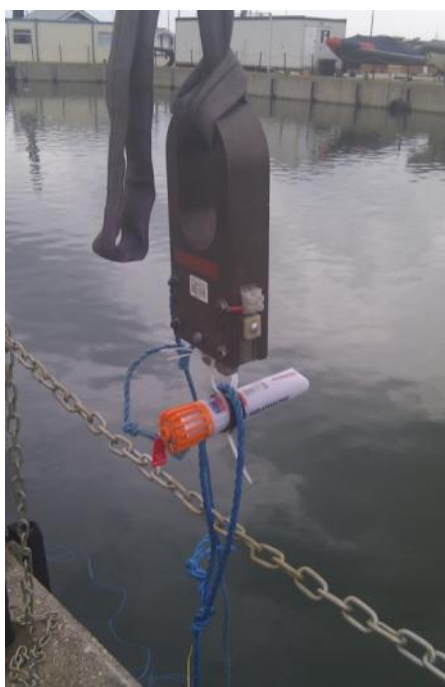
Test Set-up – Drop into Water Z501 installed in lifejacket and being hoisted by crane
