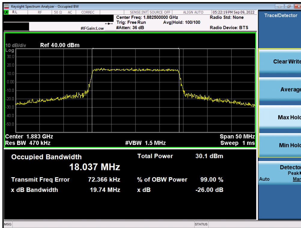
Plot 7-2. Occupied Bandwidth Plot (LTE Band 25/2 - 20MHz 16-QAM - Full RB - ANT A)
