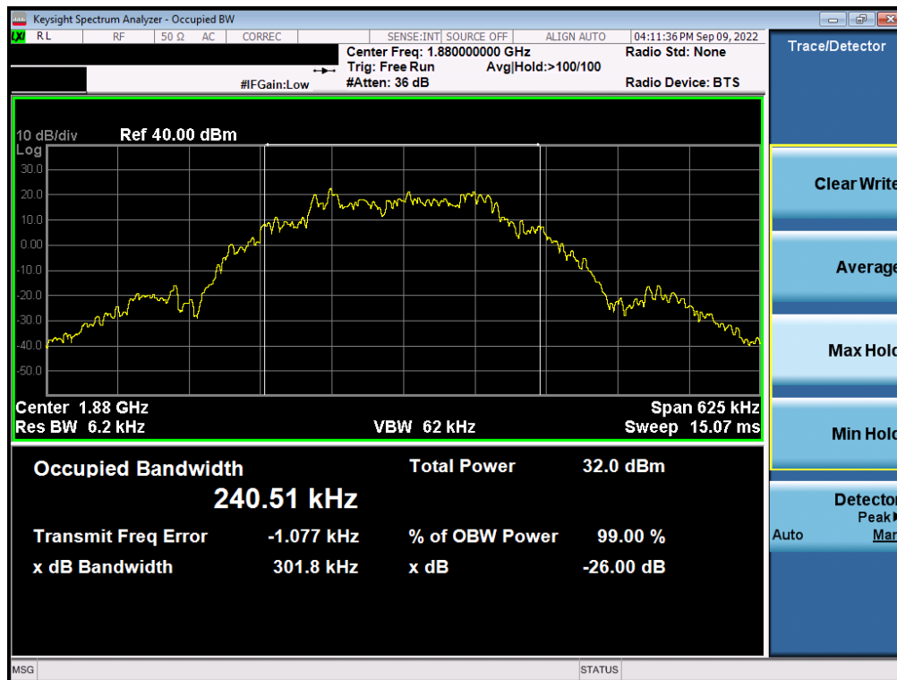
Plot 7-68. Occupied Bandwidth Plot (EDGE, Ch. 661 - ANT A)
