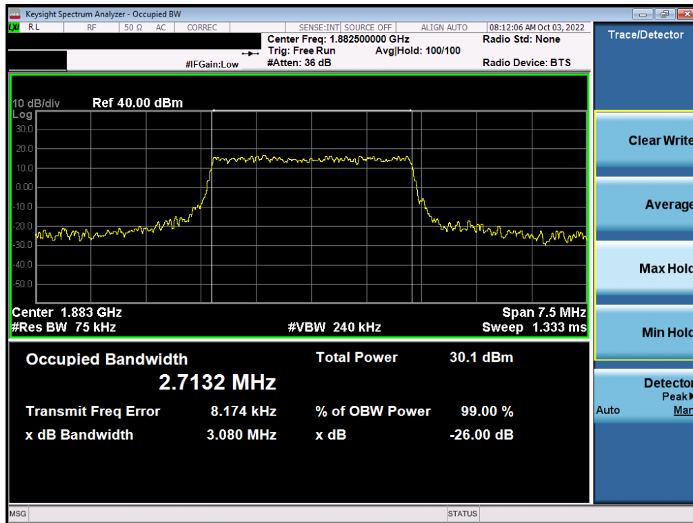
Plot 7-21. Occupied Bandwidth Plot (LTE Band 25/2 - 3MHz QPSK - Full RB - ANT F)
