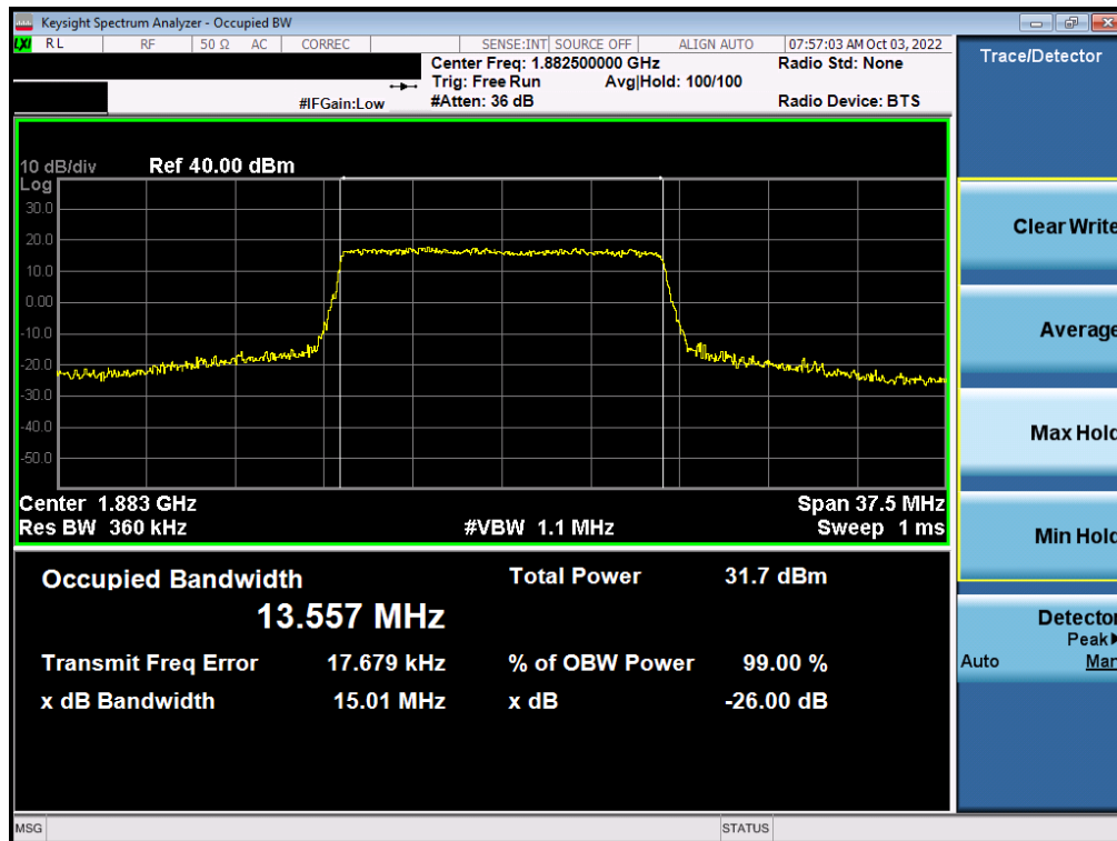
Plot 7-15. Occupied Bandwidth Plot (LTE Band 25/2 - 15MHz QPSK - Full RB - ANT F)
