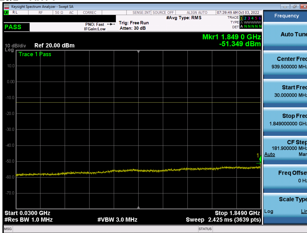
Plot 7-79. Conducted Spurious Plot (LTE Band 25/2 - 20MHz QPSK - 1RB - Low Channel - ANT F)
