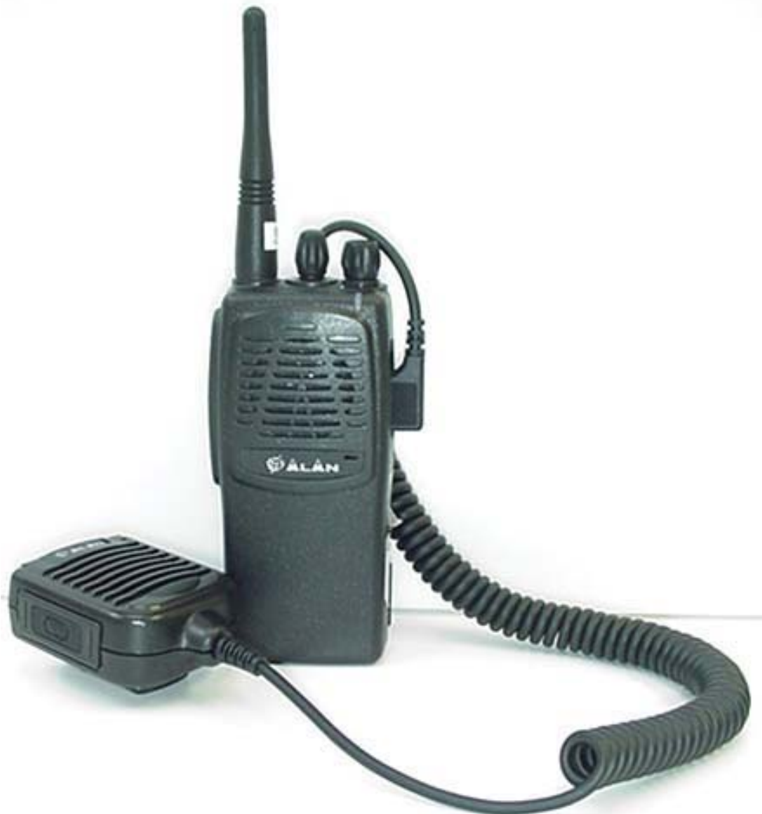
DUT with Speaker-Microphone Accessory (P/N: 70-M45WP)
