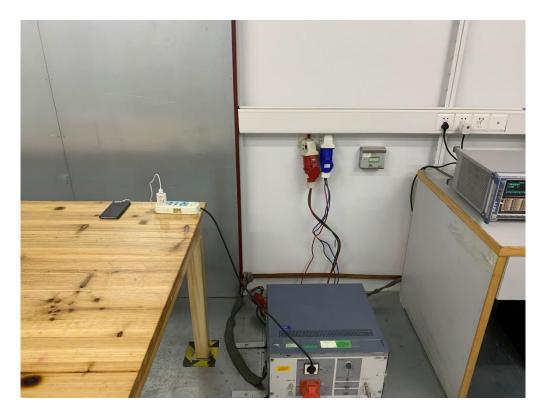
FCC RADIATED EMISSION TEST SETUP BELOW 1GHZ
