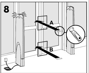
**TEST THE SYSTEM**. Hold a known good security tag horizontal and walk it through box A, stepping past the pedestals. The system should alarm.
