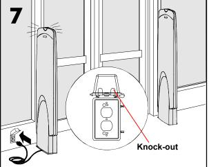
Remove the cord access knockout from the bottom of the ac receptacle guard (supplied). Replace the existing outlet cover with the receptacle guard.
