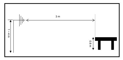
Radiated emission setup, above 1 GHz
