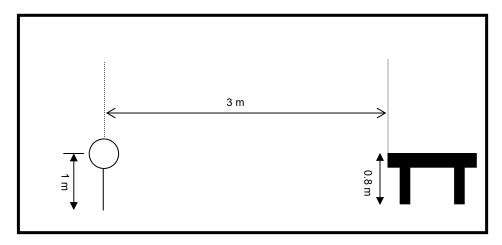
Radiated emission setup, below 1 000 MHz
