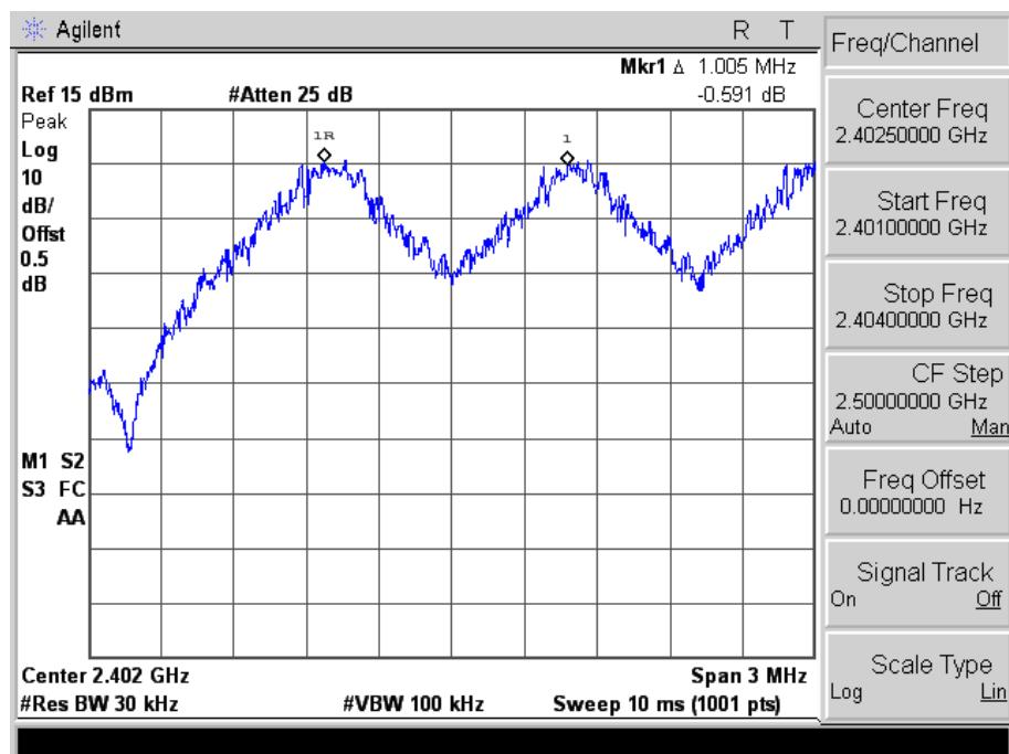
Channel Spacing (Middle CH=1MHz)
