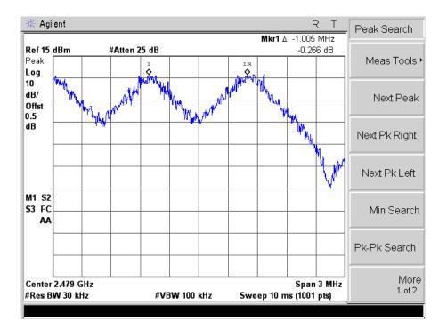
For 8DPSK mode Channel Spacing (Low CH=1MHz)
