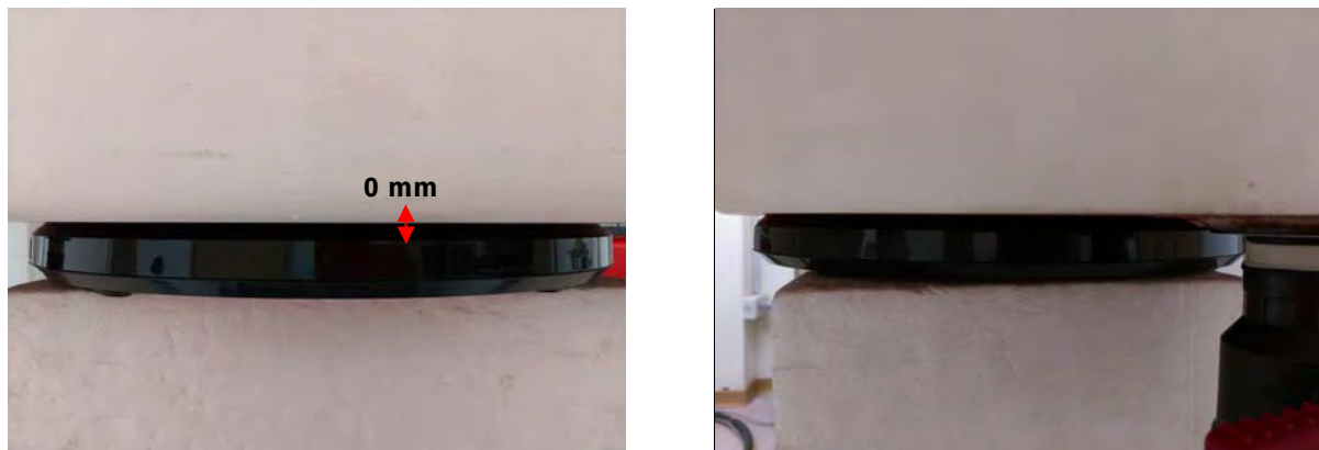
Fig.3 EUT Front side to flat phantom
