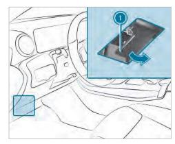
► To open: pull lever 1 to release the engine bonnet.
