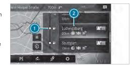
When driving on the motorway, upcoming motorway facilities 1 and available service facilities 2 are shown in the overview. These include filling stations, car parks, service stations and motorway exits, for example.
