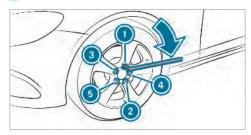
➤ Tighten the wheel bolts evenly in a diagonal pattern in the order indicated ( to s).
