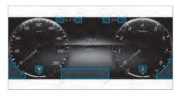
The positions of the indicator lamps on the instrument display may differ from the sample display depending on the display setting.
