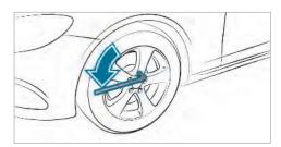
Using the wheel wrench, loosen the wheel bolts on the wheel you wish to change by about one full turn. Do not unscrew the bolts completely.
