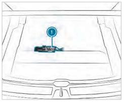
Fuse box (1) is located in the centre underneath the luggage compartment floor.
