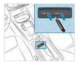
The multimedia connection unit is found in the stowage compartment under the armrest and has two USB ports. Depending on the vehicle's equipment, additional USB ports can be found in the stowage compartment of the centre console or rear folding compartment.
