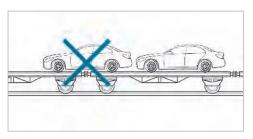
Make sure that the front and rear axles come to rest on the same transportation vehicle.
