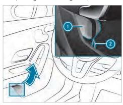
► To remove: pull out safety jacket bag ① by loop ②.
