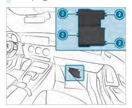
► Loosen screws ② and remove fuse box lid from the top.
