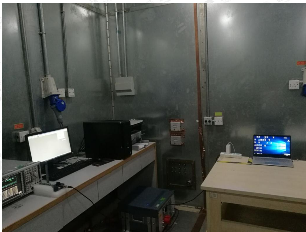
FCC RADIATED EMISSION TEST SETUP BELOW 1GHZ
