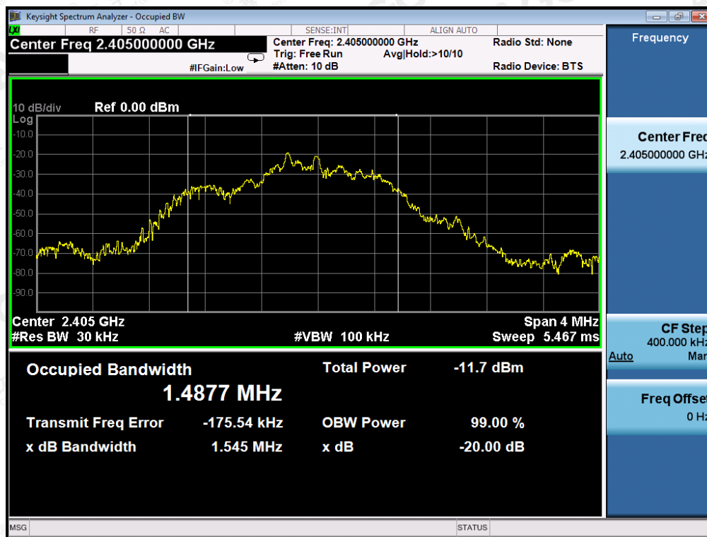
TEST PLOT OF BANDWIDTH FOR LOW CHANNEL
