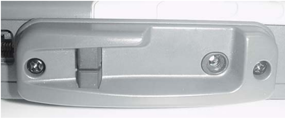
IX325 Low-Profile Hatch for AirCard 860 PCMCIA Card (Antenna Removed)
