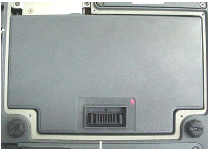
Internal Li-ion Battery 11.1 V, 3600 mAh (Model: T8M-E)
