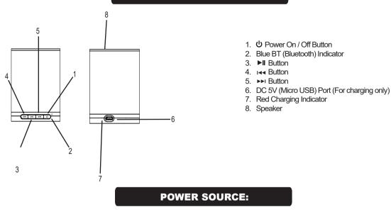
The unit has a built-in Li-ion rechargeable battery, recharge it before first time use or when it is drained as follow:
