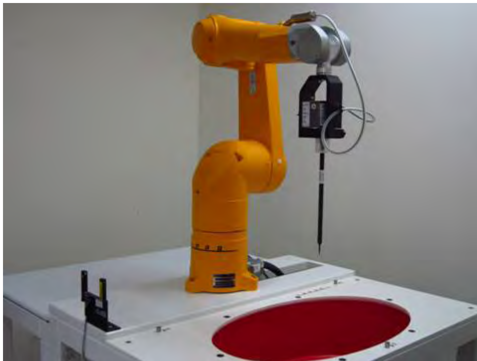
Fig.1 Photograph of the SAR measurement system
