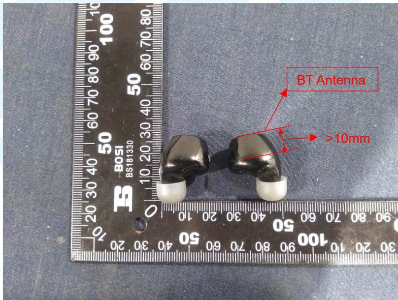
The minimum contact distance is more than 10 mm. So, the 10 mm separation distance applies.
