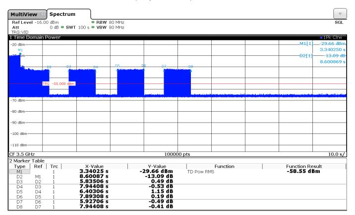
Note: The higher emissions are belonging to the companion device, the lower emissions are the transmissions of the EUT.
